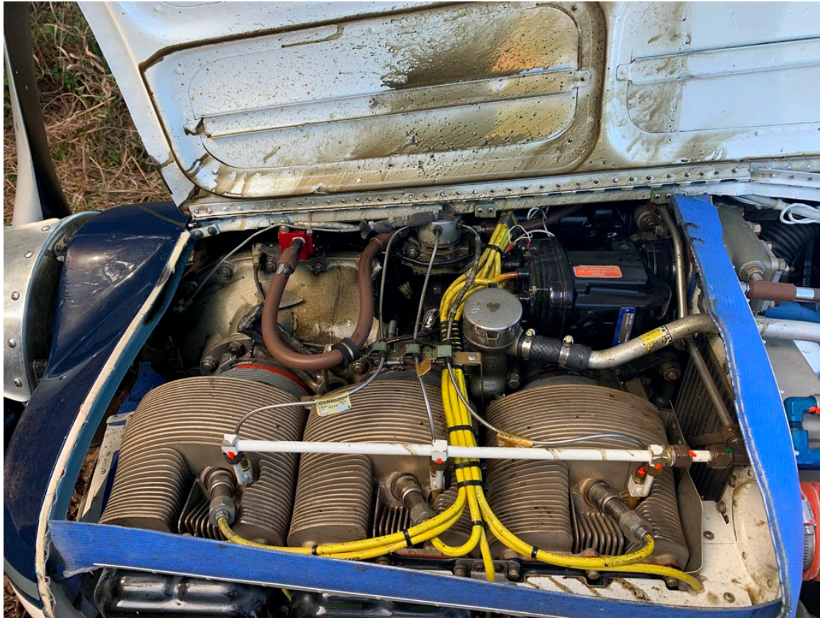
Photograph 5 - View of Engine and Damage to the Engine Case (Courtesy of Pierce County Fire Department)
