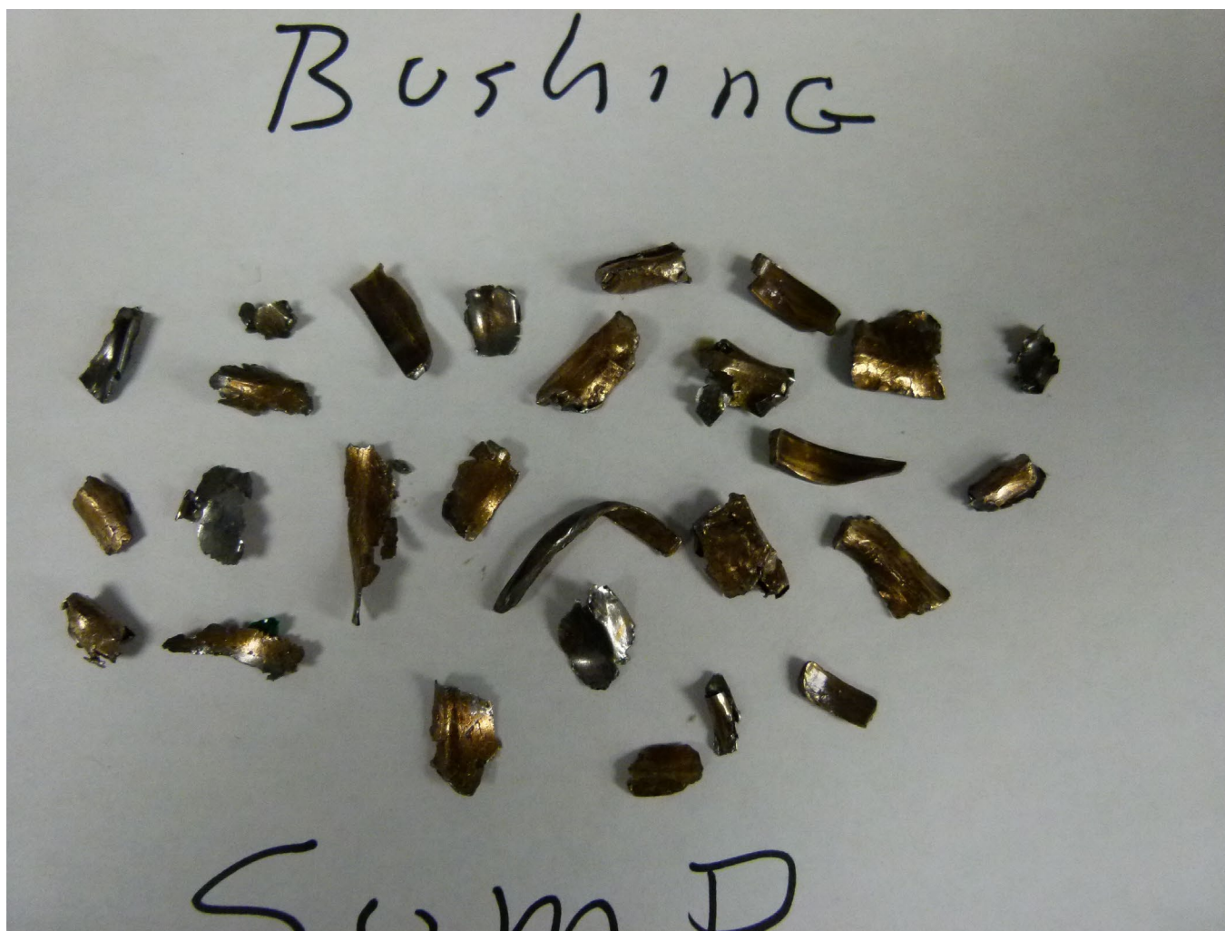
Photograph 7 - Bushing pieces discovered in sump. (Courtesy of Continental Engines)
