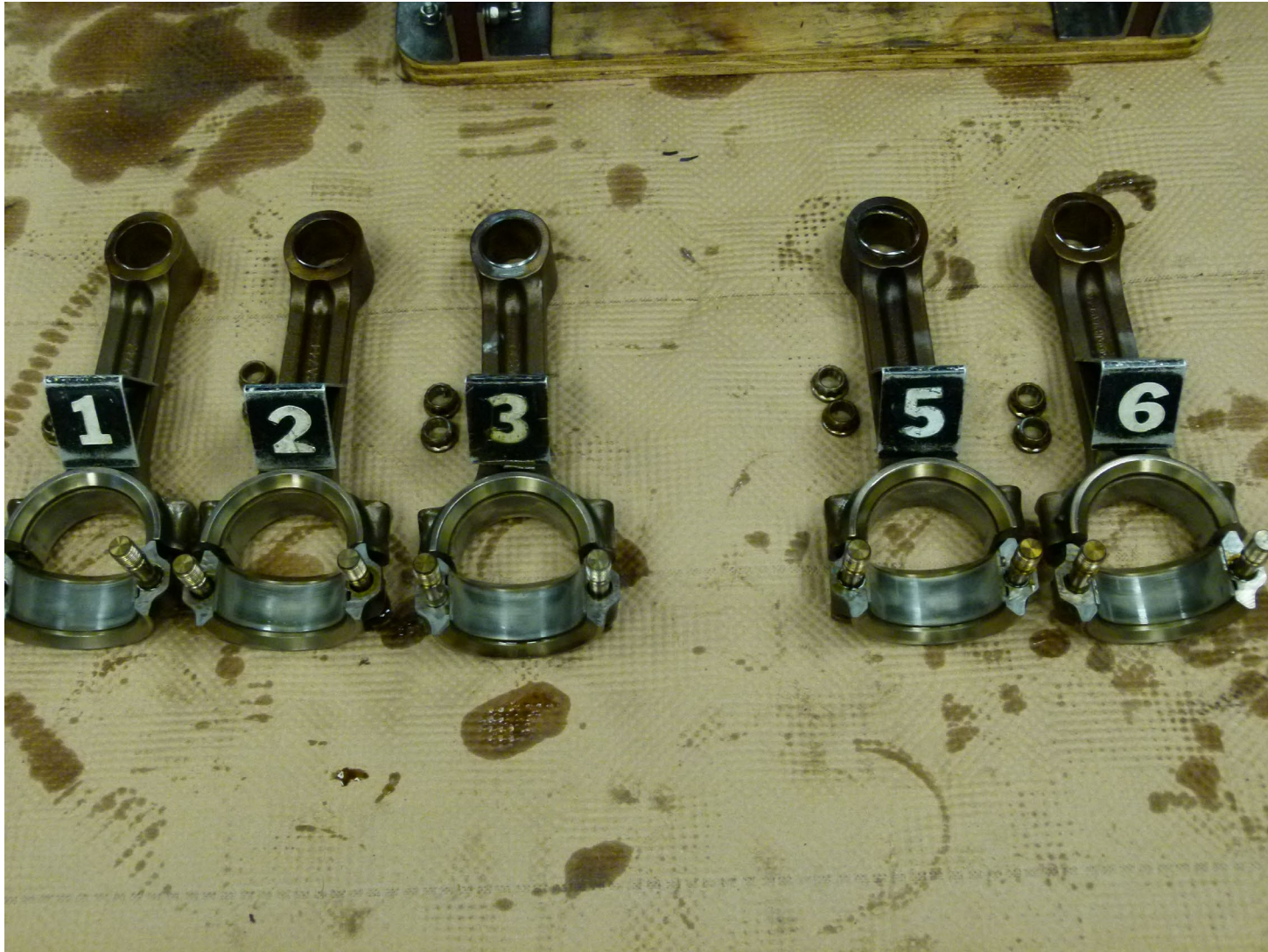
Photograph 5 - Remaining piston rods and bushings. (NTSB)
