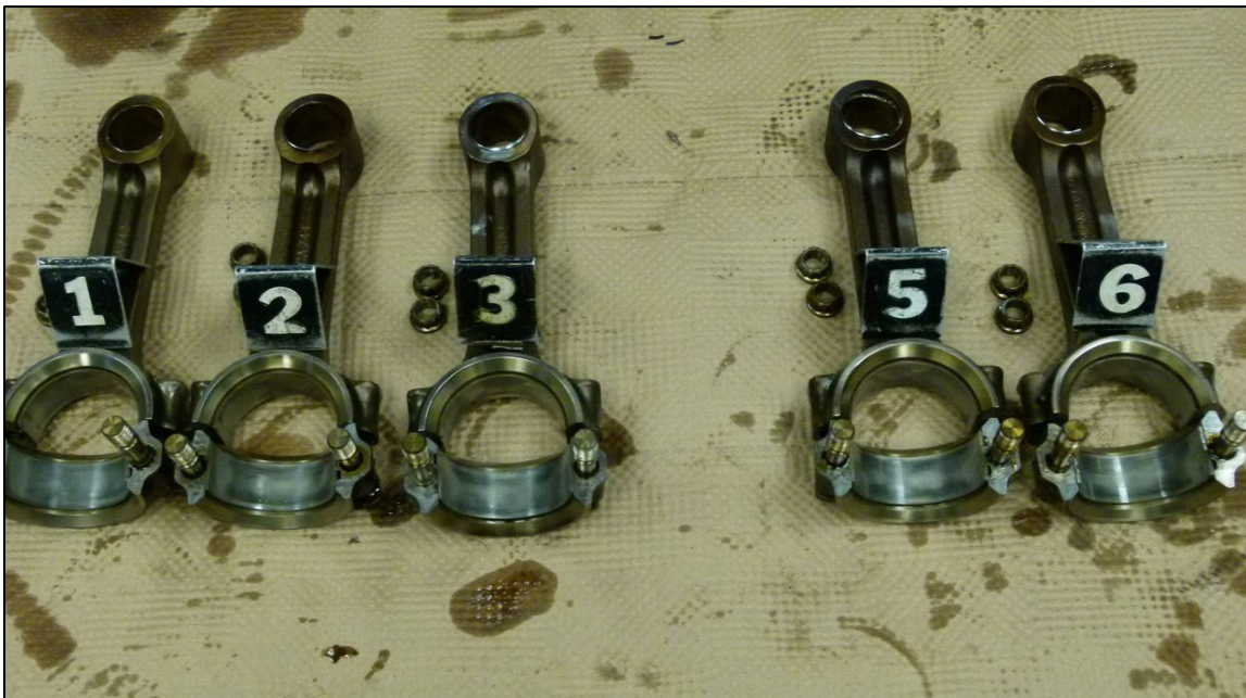
Figure 3 Connecting rod assemblies minus the number 4 that was destroyed.
