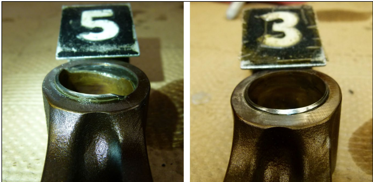
Figure 4 Close up of connecting rod bushings migration and damage. This is indicative of all remaining rods and their respective bushings.
