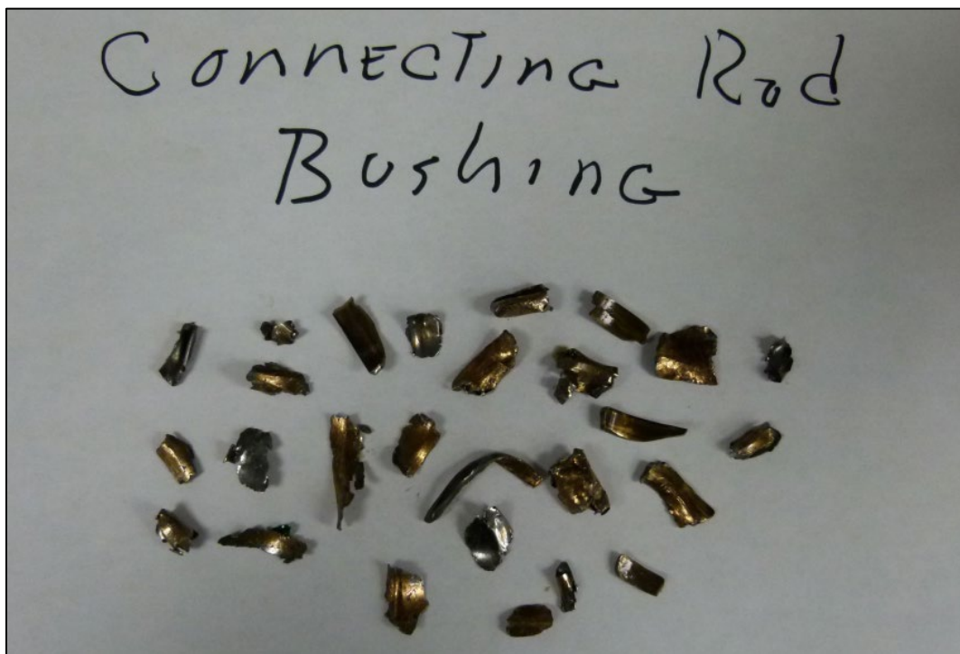
Figure 5 The number 4 connecting rod bushing discovered in sump and crankcase.
