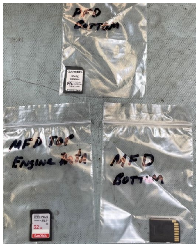
Figure 2. Garmin G1000 SD cards as received by the NTSB Vehicle Recorder Laboratory.
