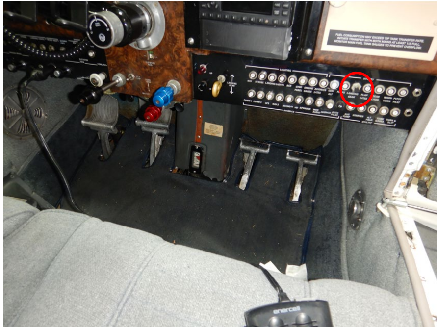
Pulled Landing Gear Breaker (Courtesy of Textron Aviation)
