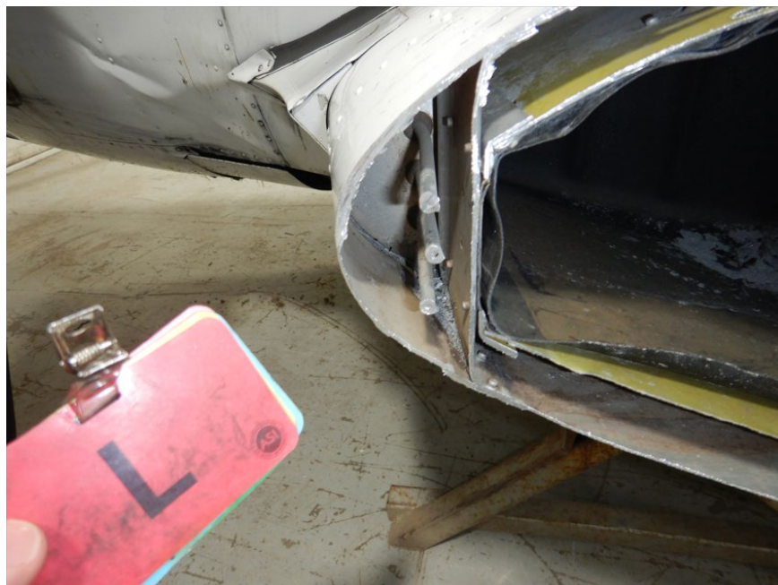
Fuel Lines and Vents on Left Side (Courtesy of Textron Aviation)
