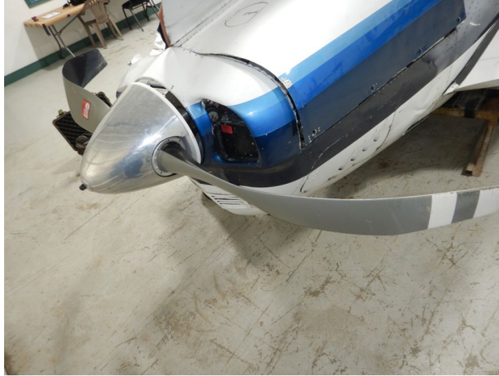
Damage to Propeller (Courtesy of Textron Aviation)
