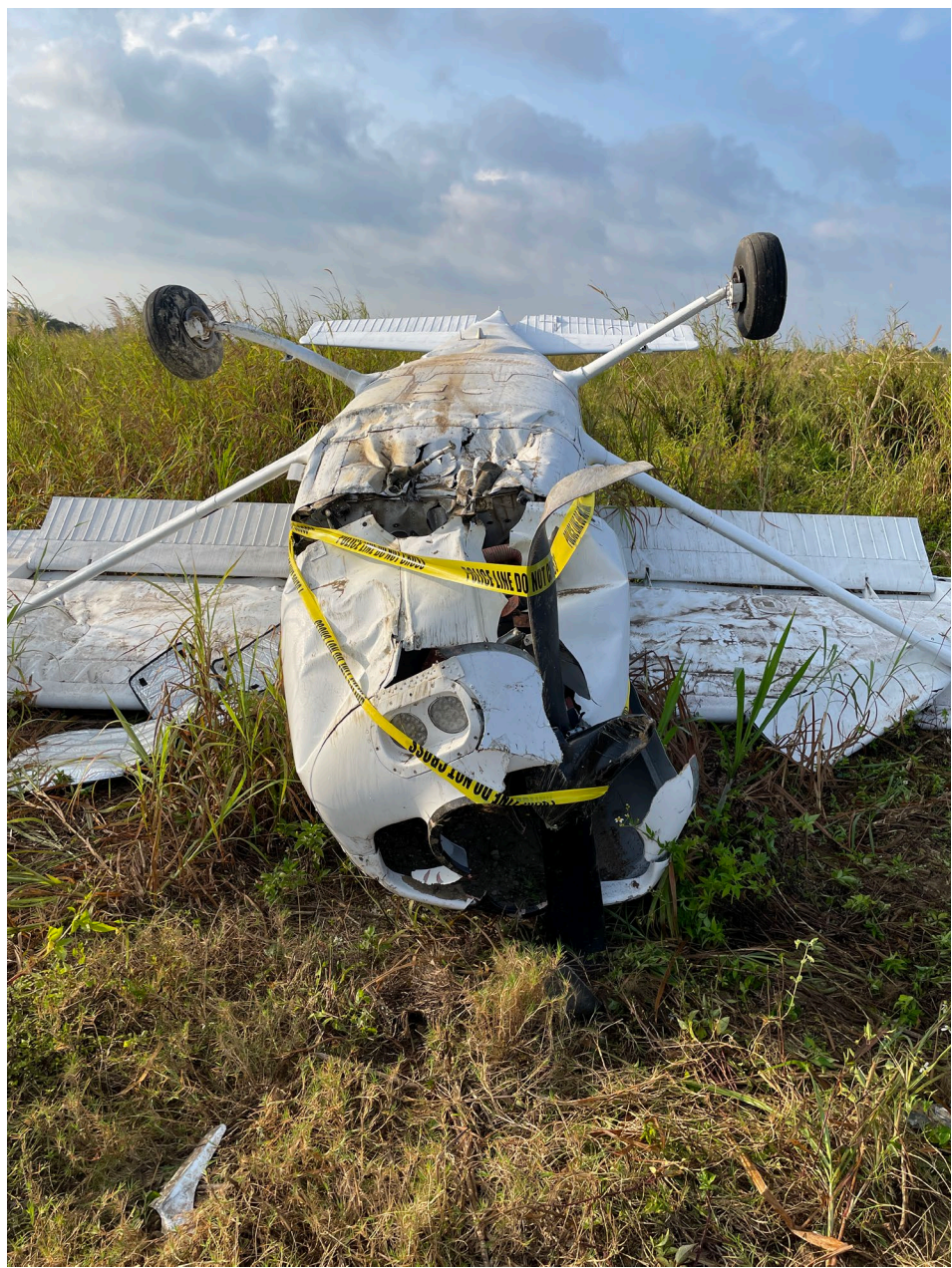
Photo 2 – Close up view of fuselage and wing damage.
