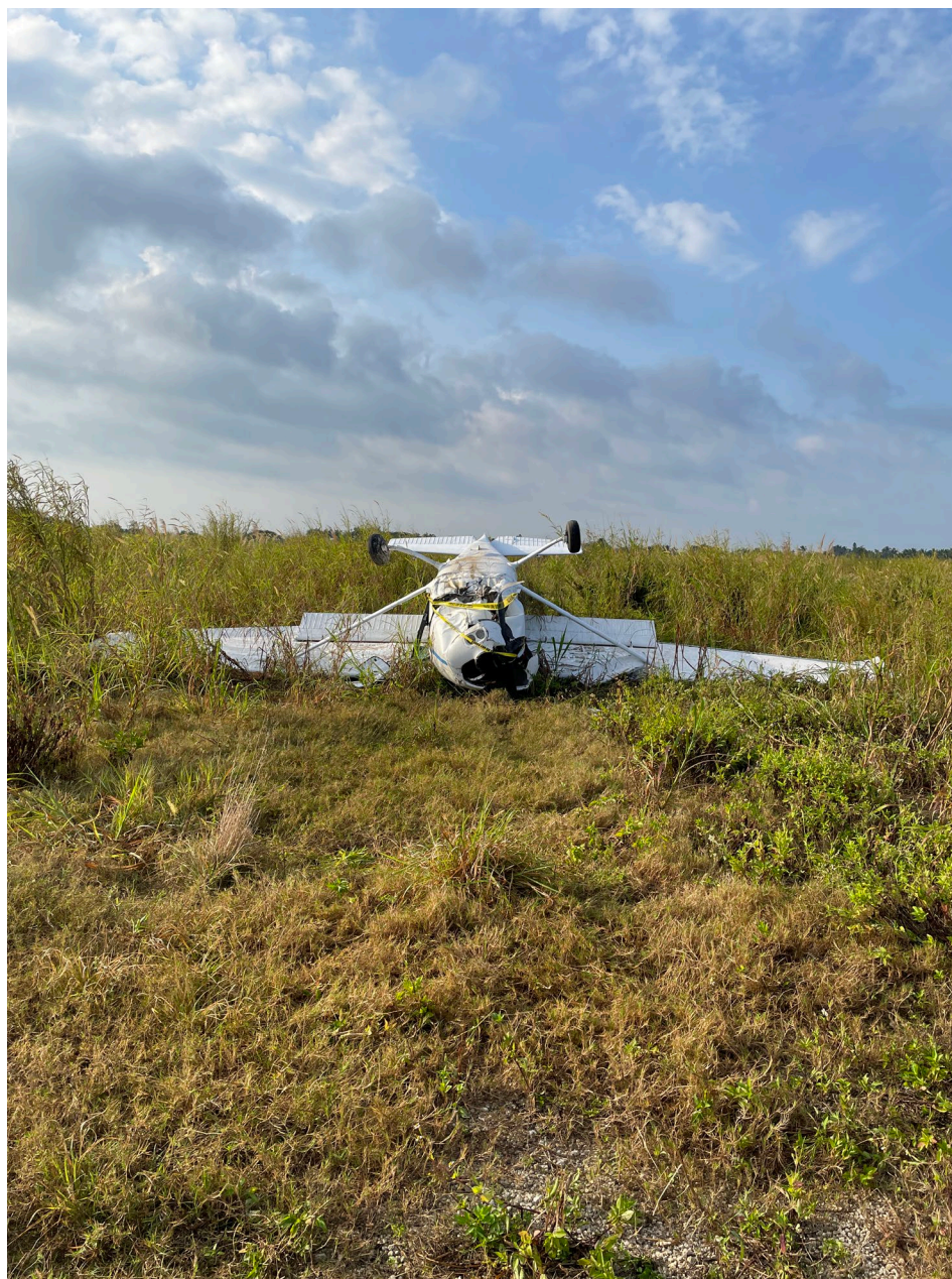
Photo 1 – Forward view of airplane upside down showing airframe buckling
