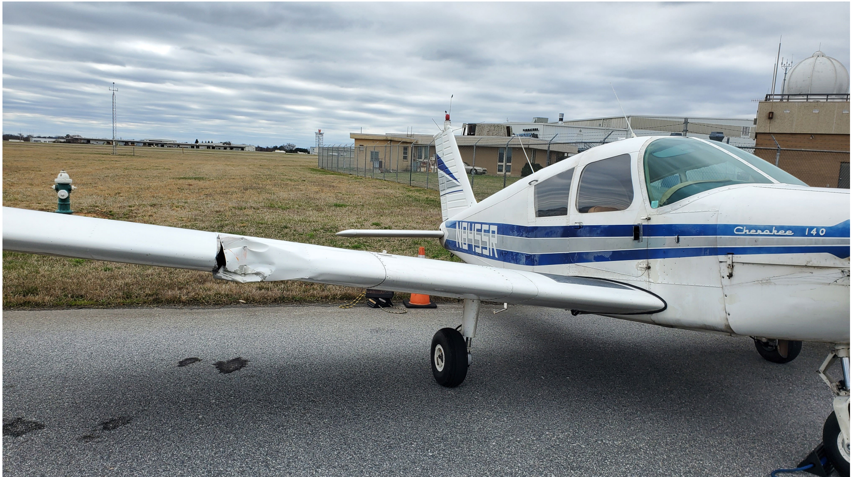
Photograph 1 - Damaged right wing. (courtesy of FAA)
