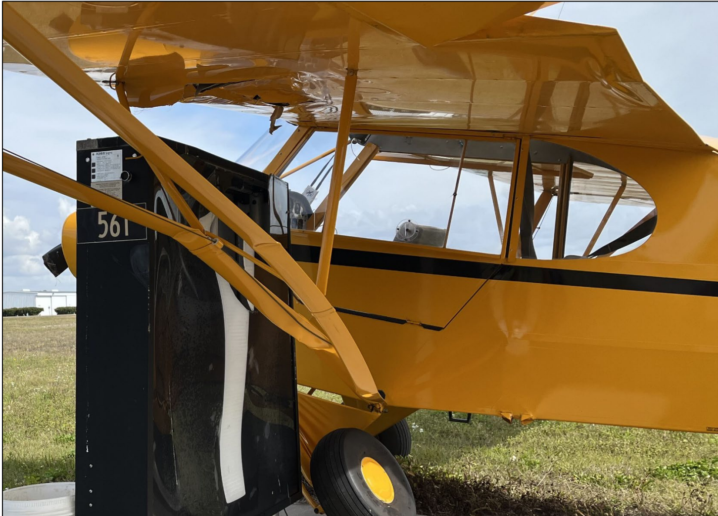
Photo 2: View of wing strut and wing root damage (Photo Courtesy of FAA)
