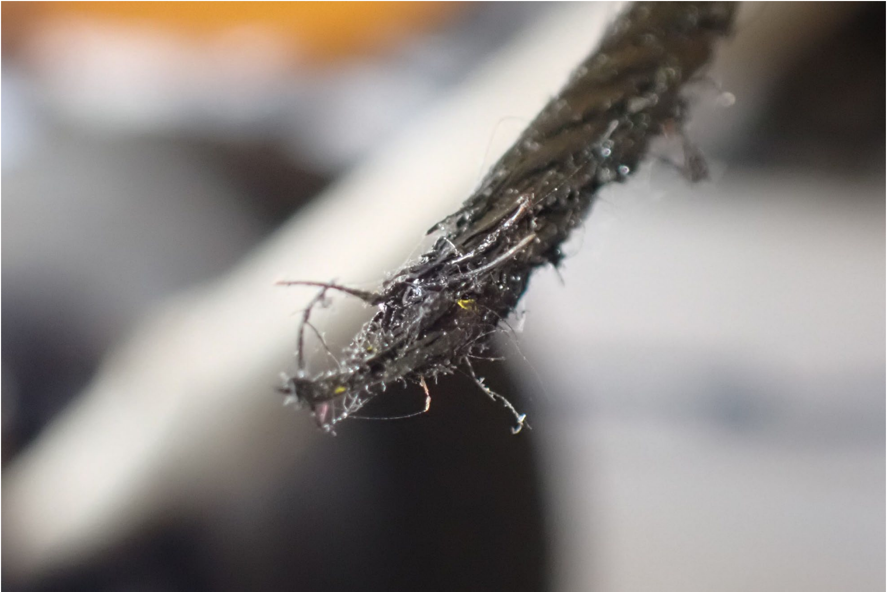
Photograph 4 - Broken aileron cable at fuselage
