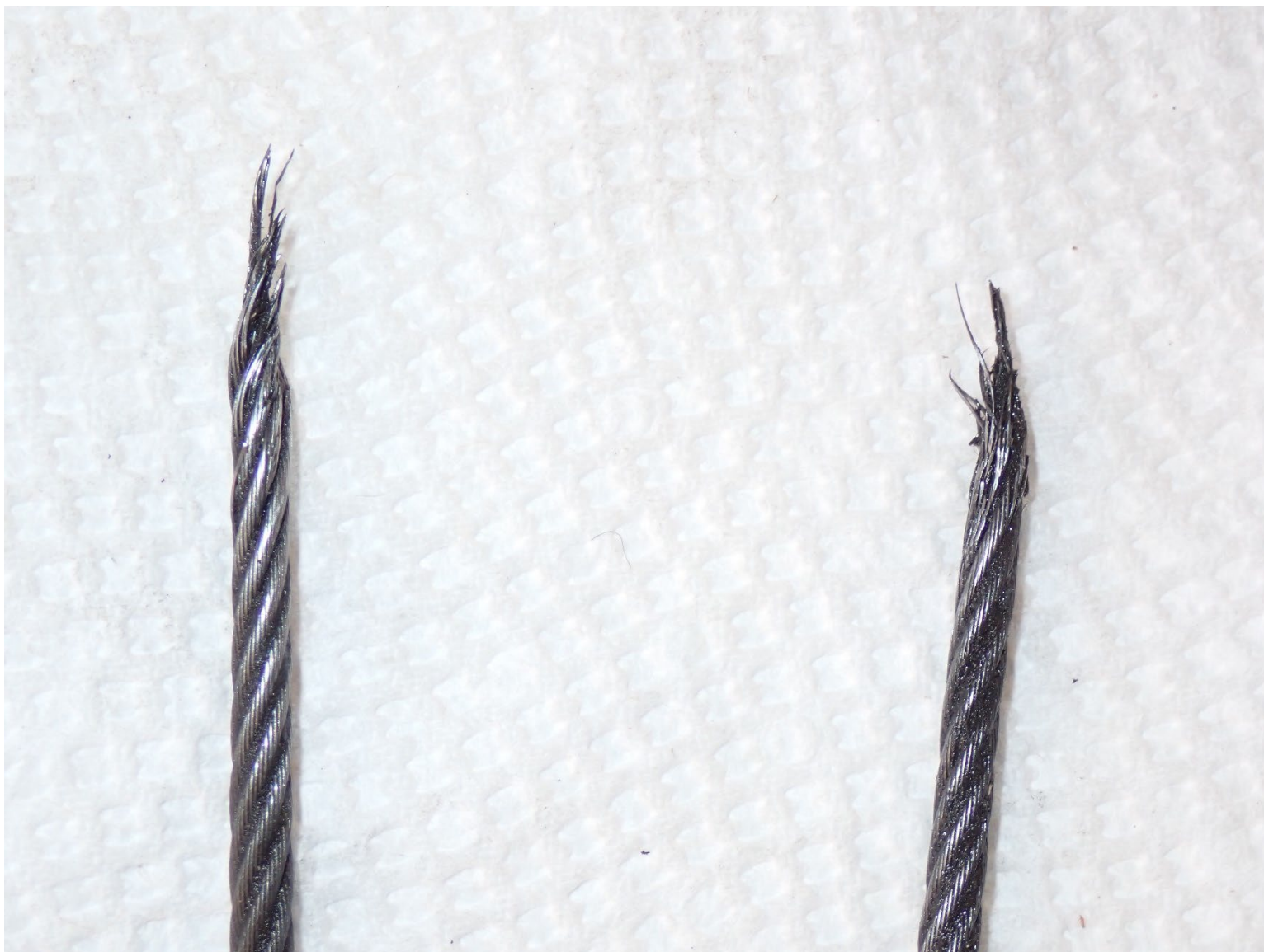
Photograph 7 - Close up view of broken aileron cable
