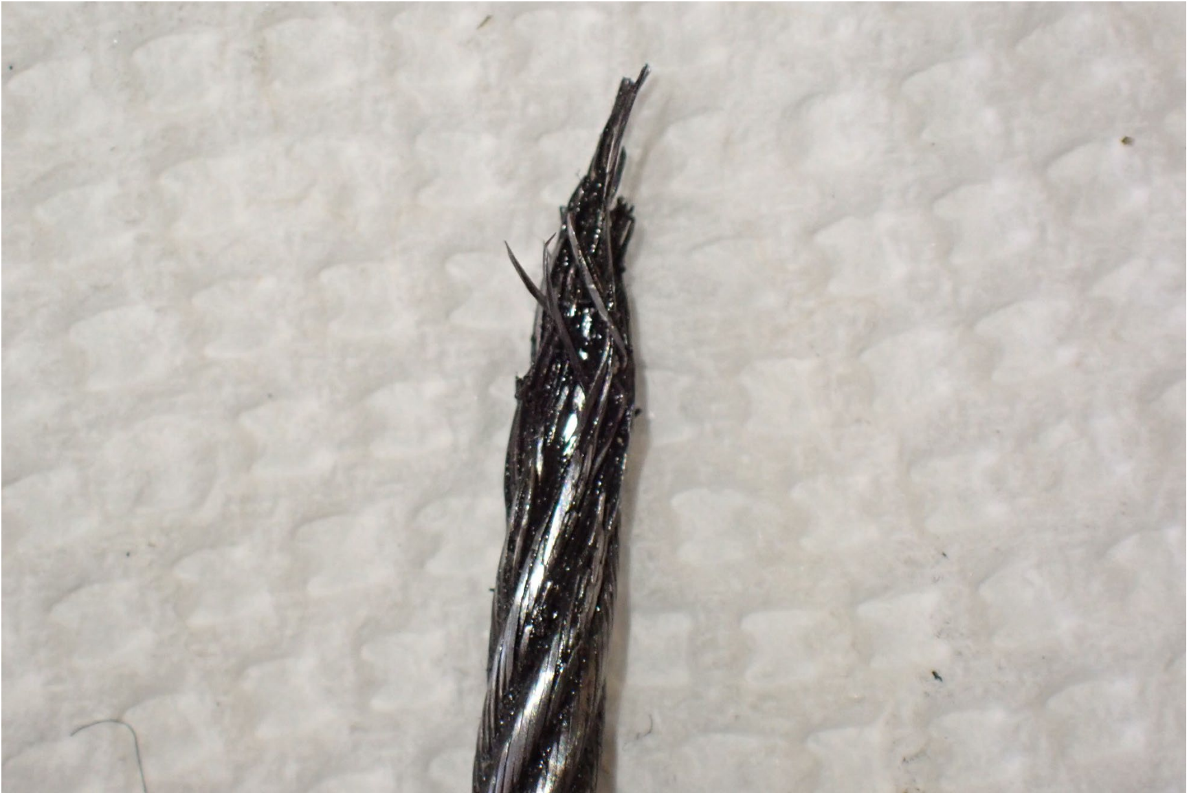
Photograph 8 - Close up view of broken aileron cable (fuselage side)
