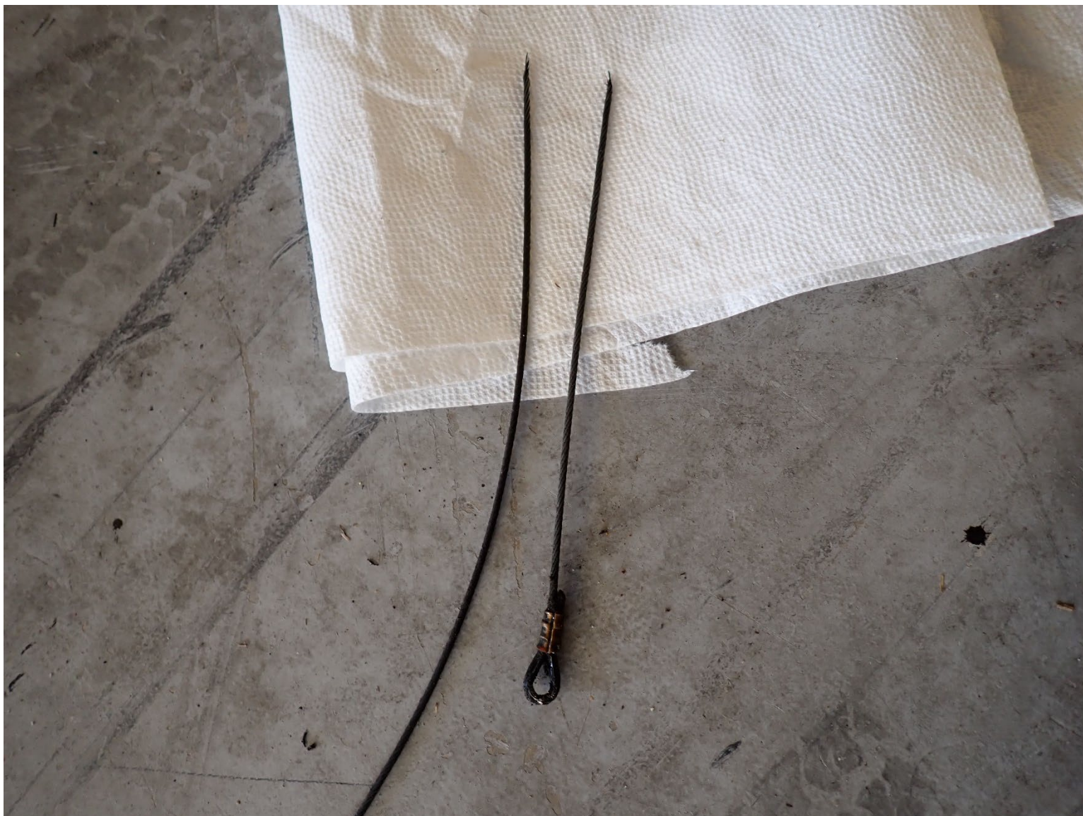
Photograph 6 - Both sides of the broken aileron cable
