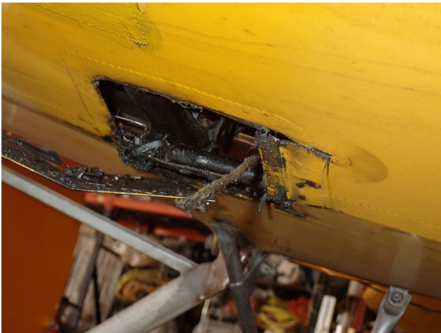
Photograph 3 - Broken aileron cable at fuselage
