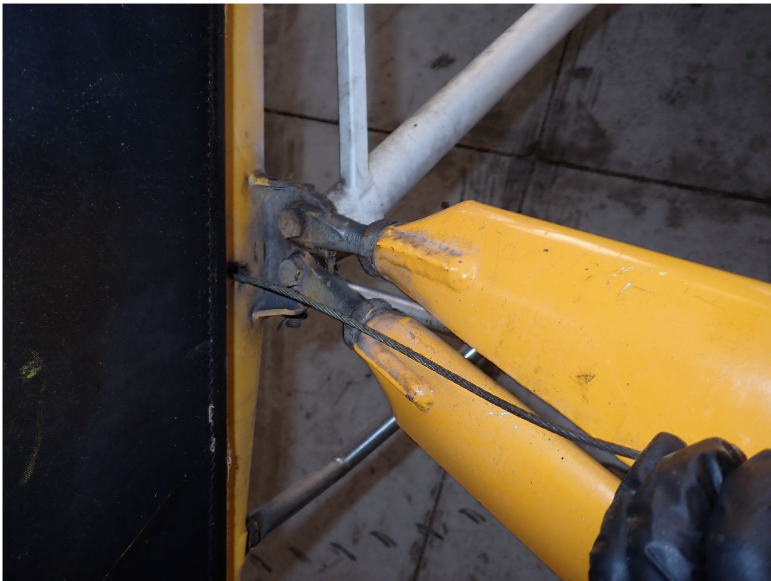
Photograph 14 - Right direct aileron cable at the lower right fuselage pulley
