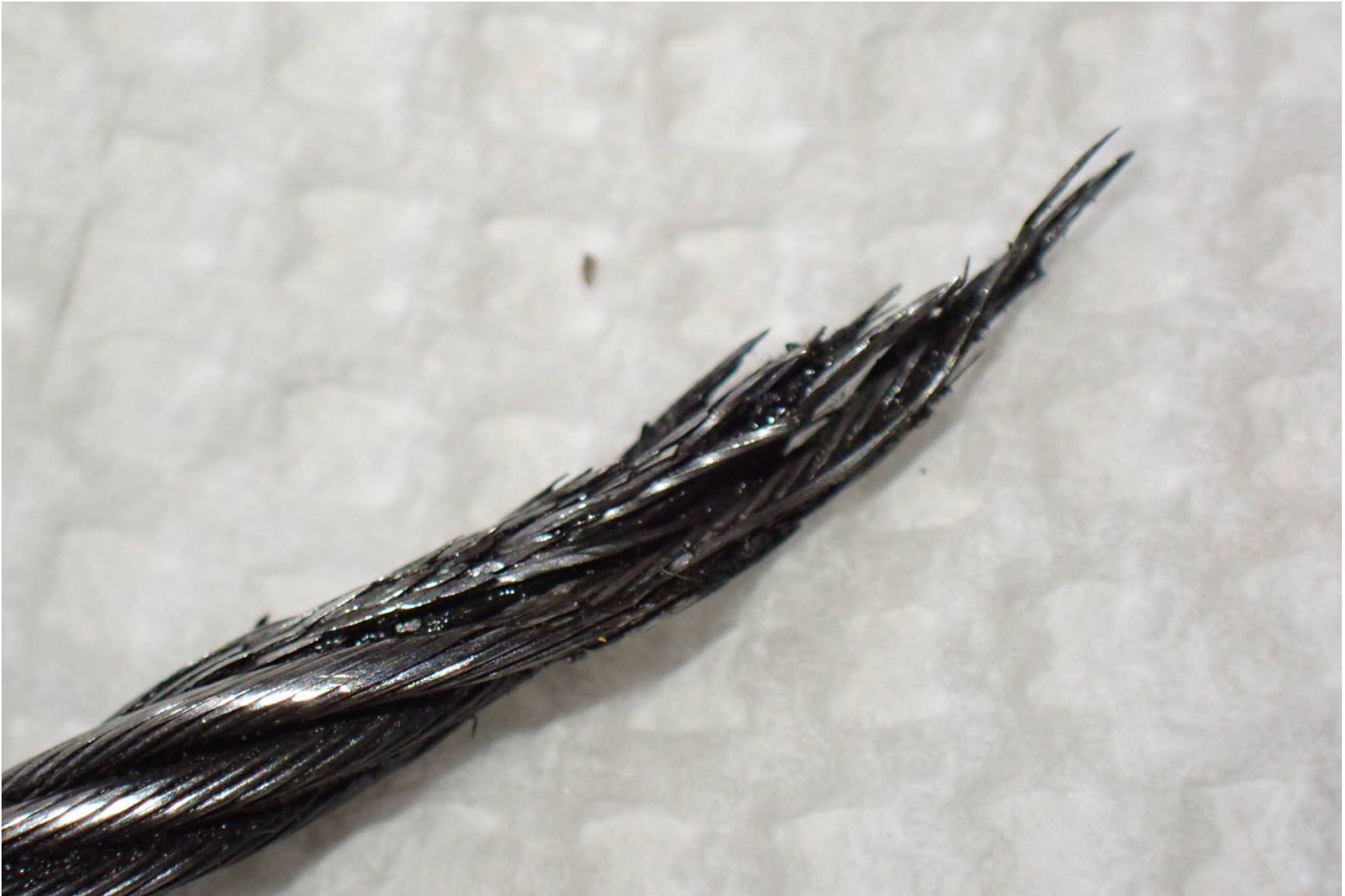
Photograph 9 - Close up view of broken aileron cable (aileron side)
