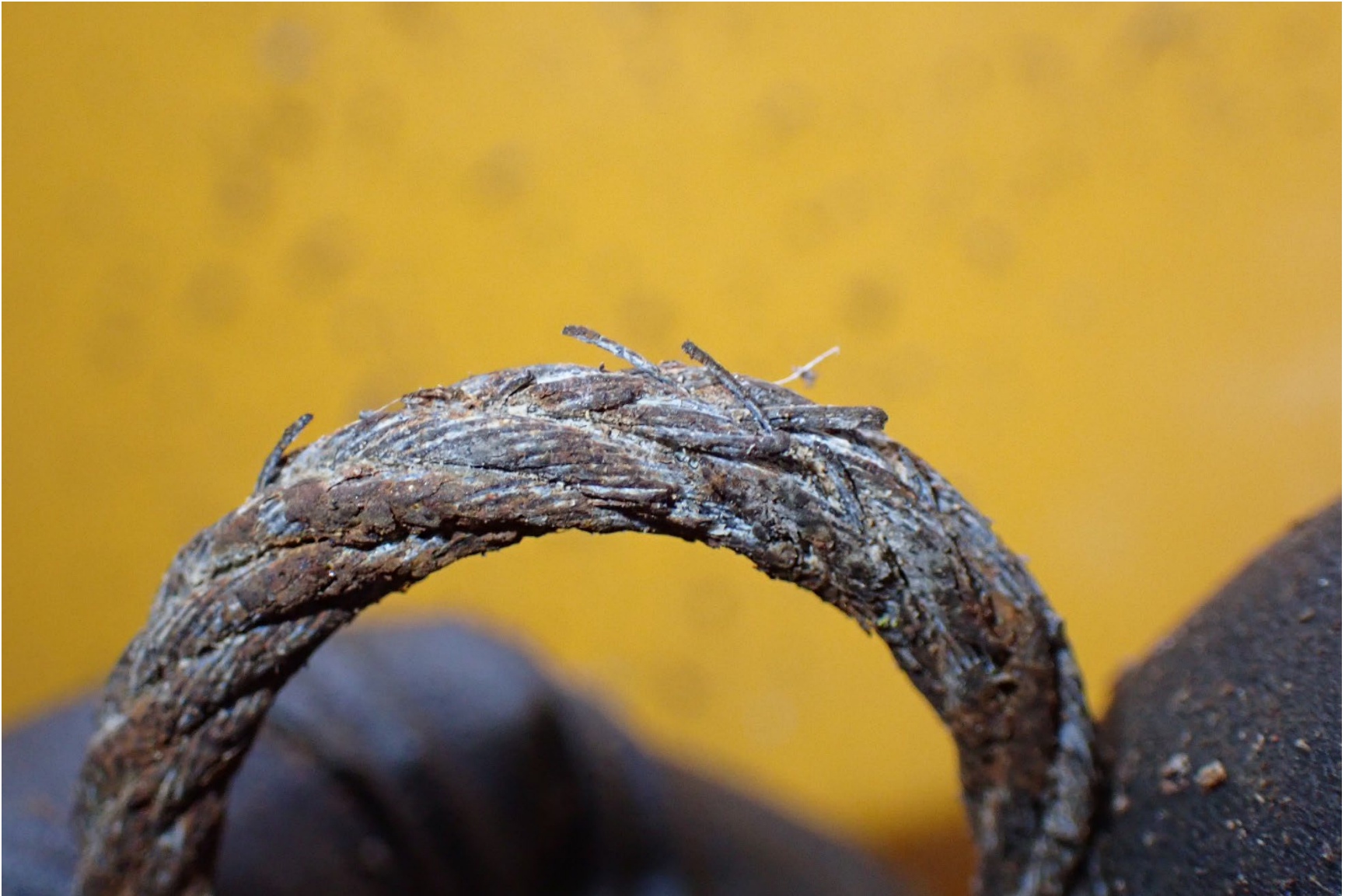
Photograph 16 - Corrosion and broken strands on the right direct aileron cable
