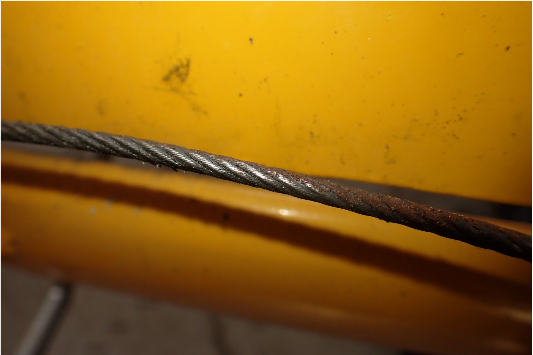
Photograph 15 - Corrosion and wear on the right direct aileron cable
