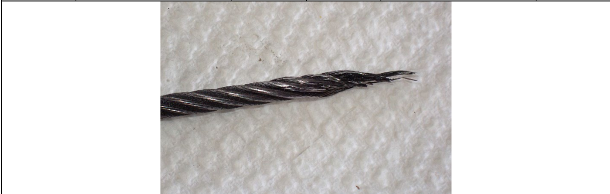
Figure 5: Fractured end of the left aileron direct cable (aileron side of the cable)
