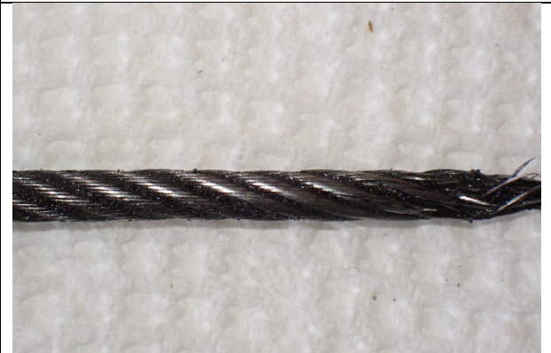
Figure 4: Wear spots on left aileron direct cable (control stick side of the cable)
