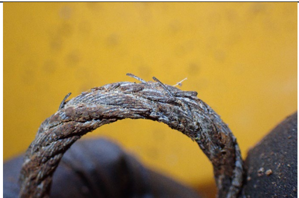
Figure 10: Right aileron direct cable with visible corrosion and broken wire strands
