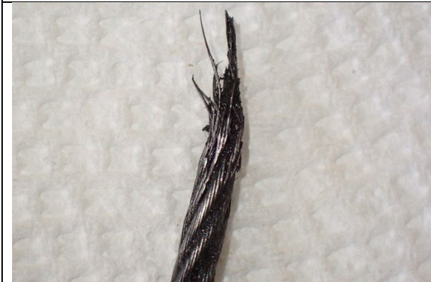
Figure 3: Fractured end of left aileron direct cable (control stick side of the cable)
