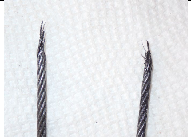
Figure 2: Both fractured ends of the left aileron direct cable
