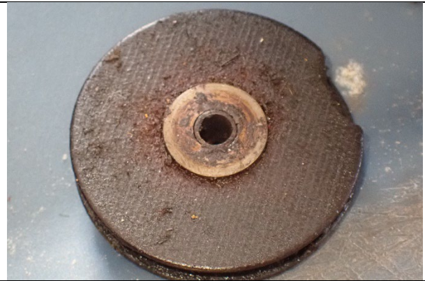
Figure 7: Left aileron direct cable pulley with visible corrosion
