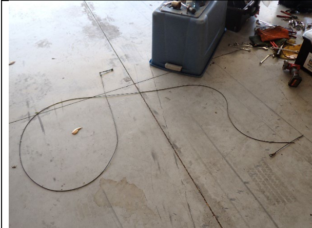
Figure 1: Both sides of the fractured left aileron direct cable
