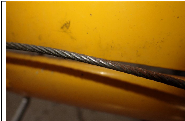
Figure 9: Right aileron direct cable with visible corrosion and wear marks
