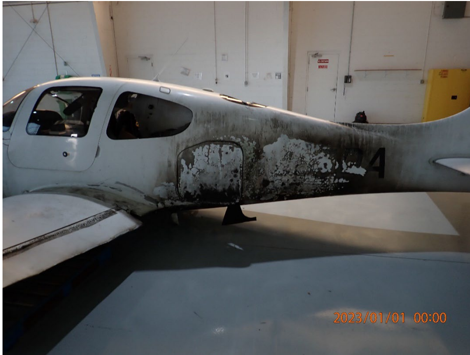
Thermal Damage to the Fuselage
