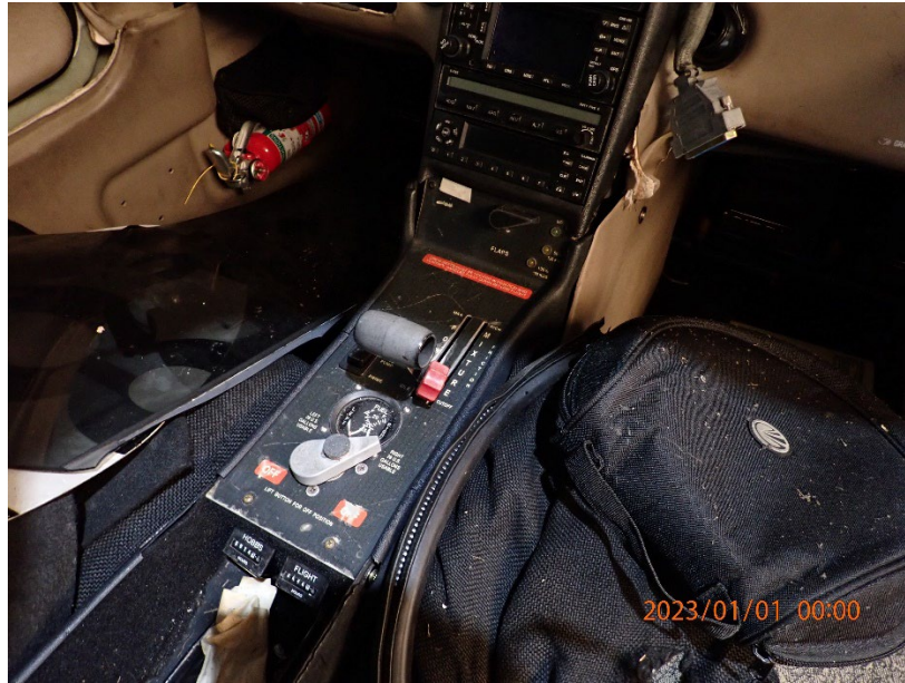
Fuel Controls as Found
