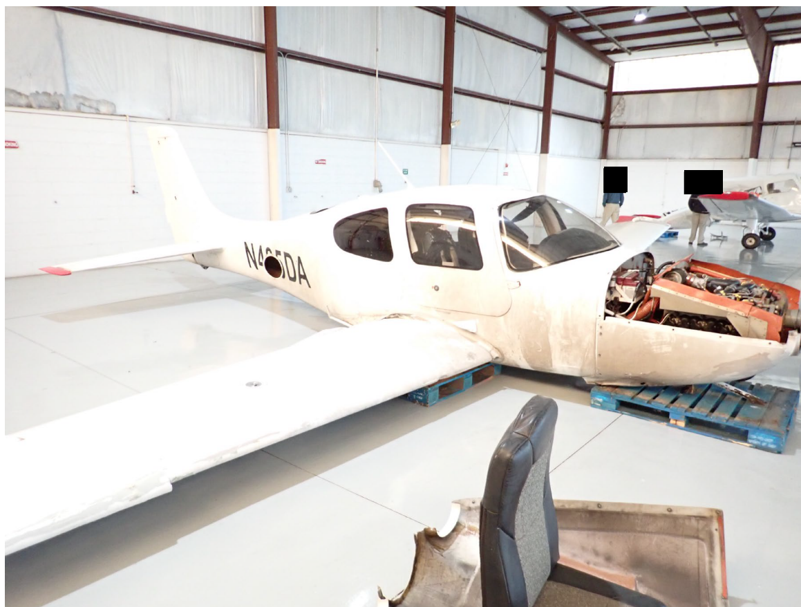
Photograph 3 - Airplane Right Side Damage
