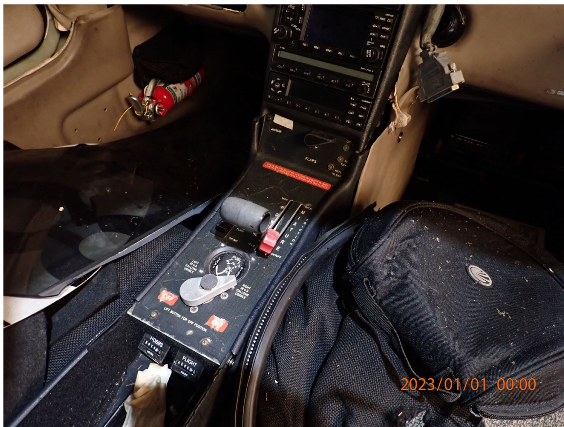
Photograph 4 - Fuel Controls as Found
