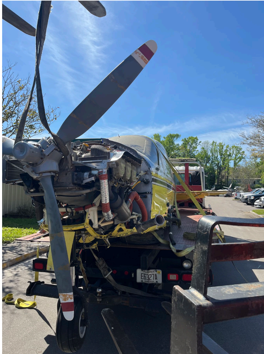
Photograph 5 - Airplane Test Run Set-up with Test Propeller
