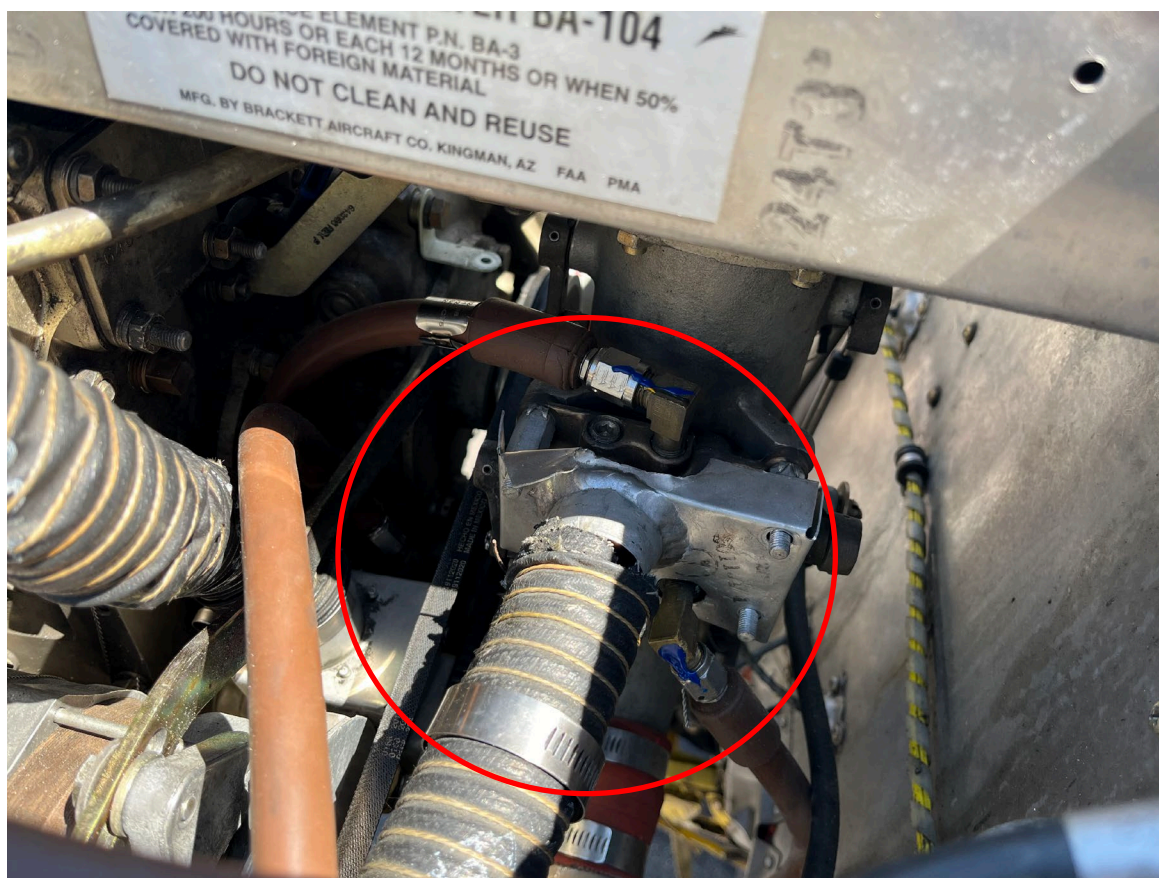
Photograph 2 - Location of the Leaking Fuel
