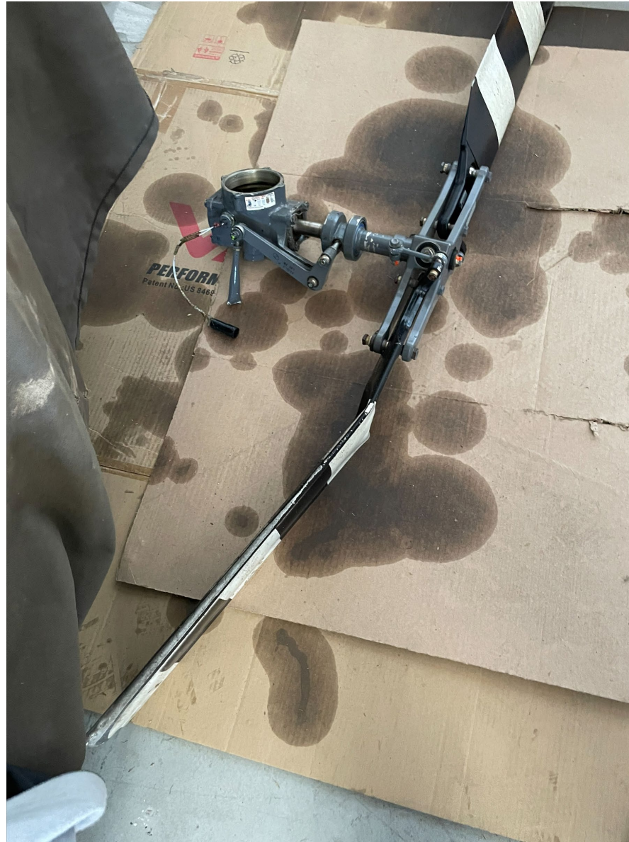
Photograph 3 - Fractured tail rotor
