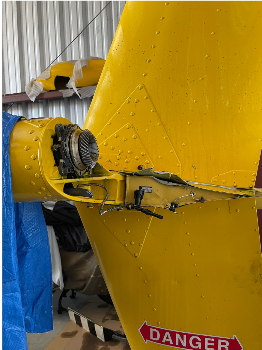
Photograph 1 - Tail rotor assembly with fracture tail rotor.
