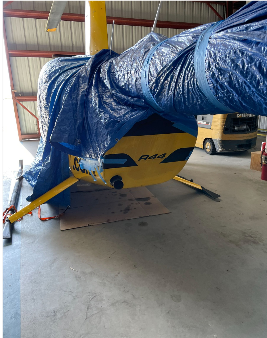
Photograph 2 - Helicopter with displaced skids
