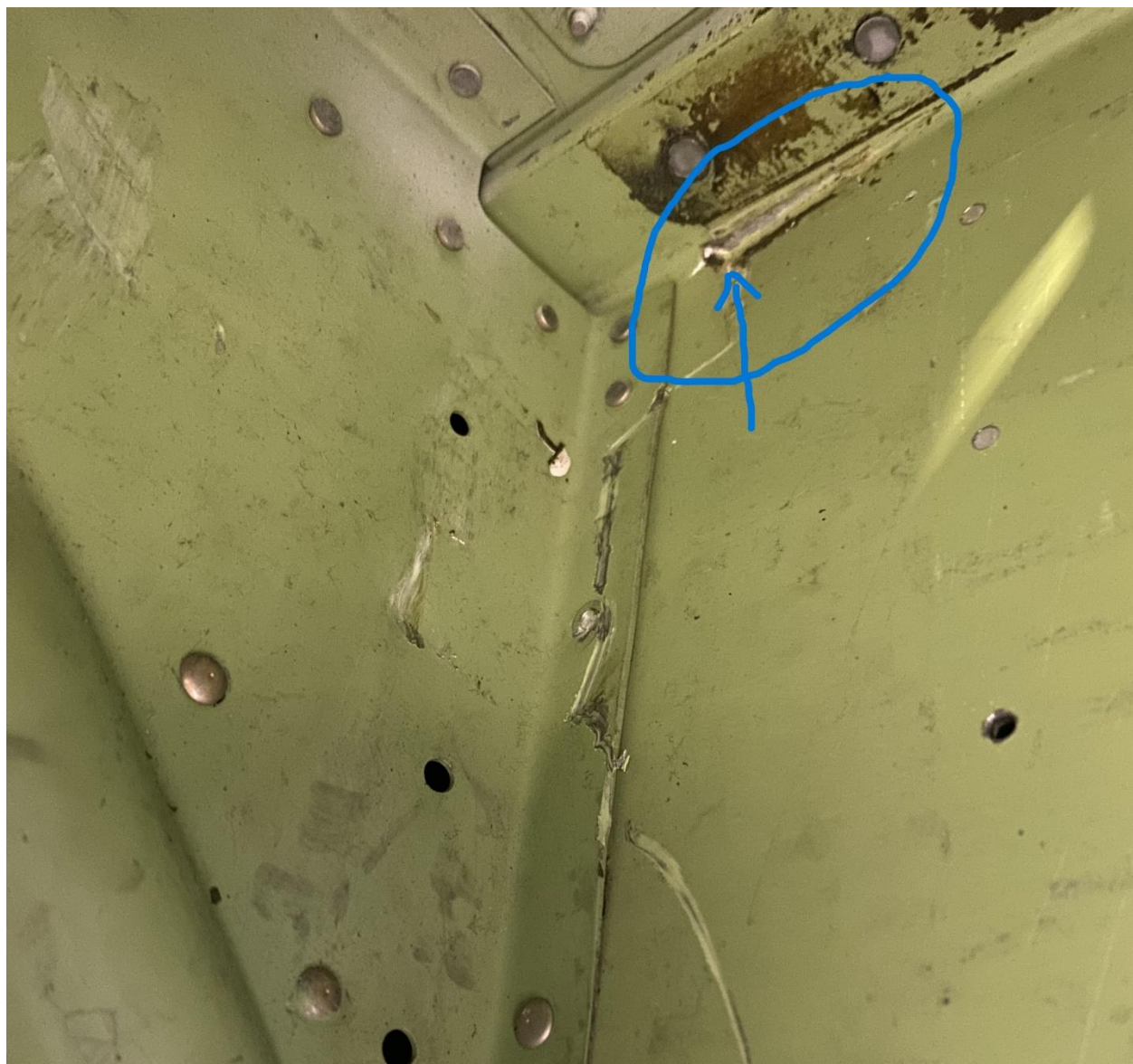
Photograph 4 - Crack found in the right-wing structure (Courtesy of FAA)
