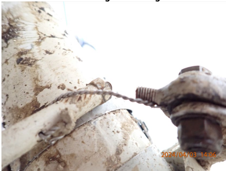
Fractured Right Hand Lower Steering Rod
