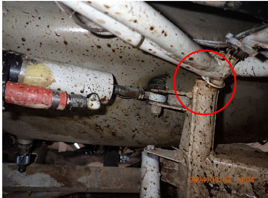
Damage to the Upper Leg of the Nose Gear
