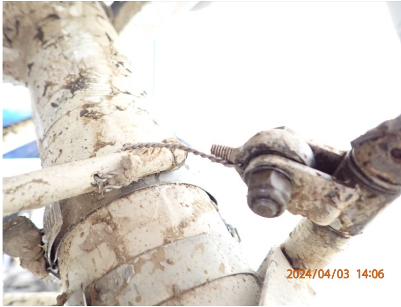
Fractured Right Hand Lower Steering Rod
