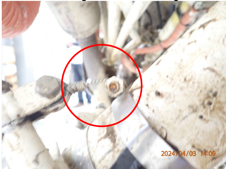
Fractured Right Hand Lower Steering Rod
