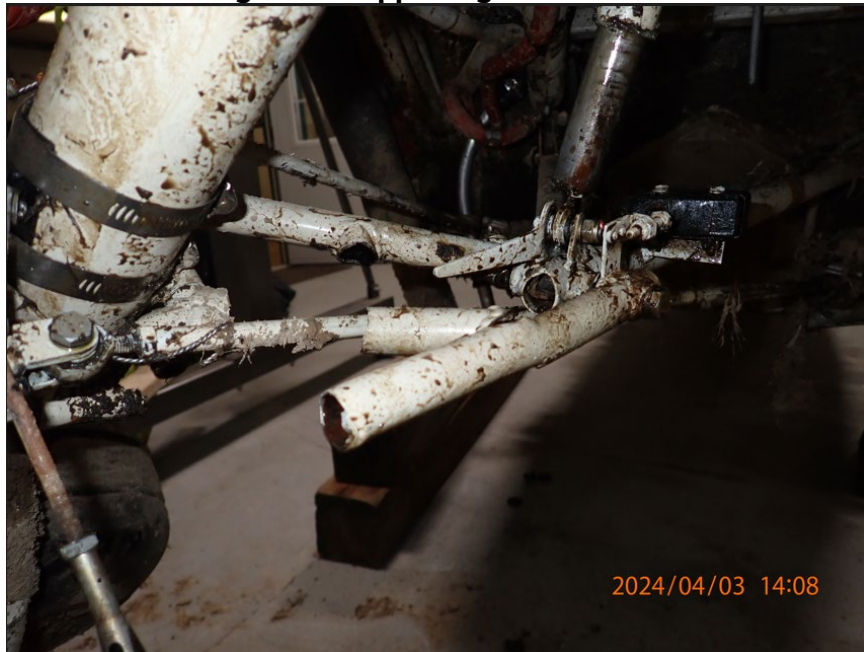
Lower Drag Strut Damage
