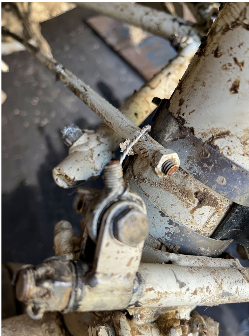
Photograph 3 - Broken Right-Hand Lower Steering Rod
