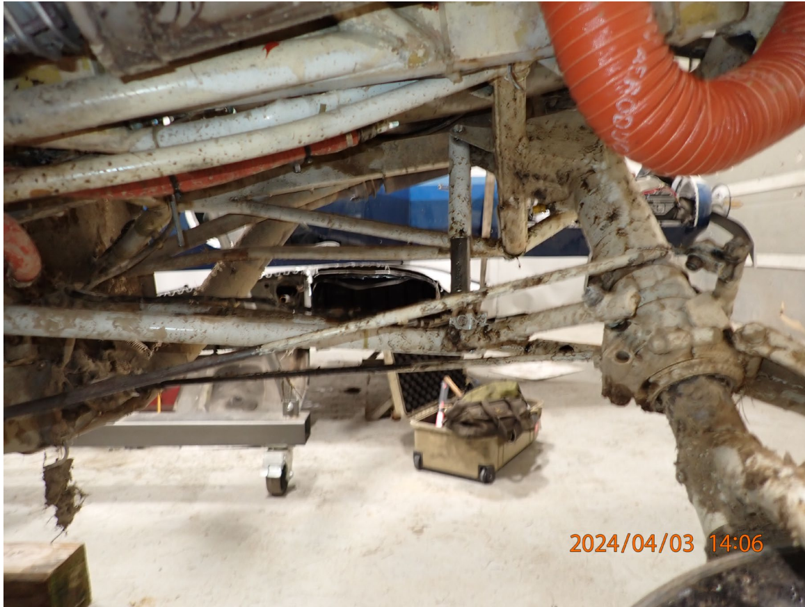
Photograph 2 - Damage to Nose Gear
