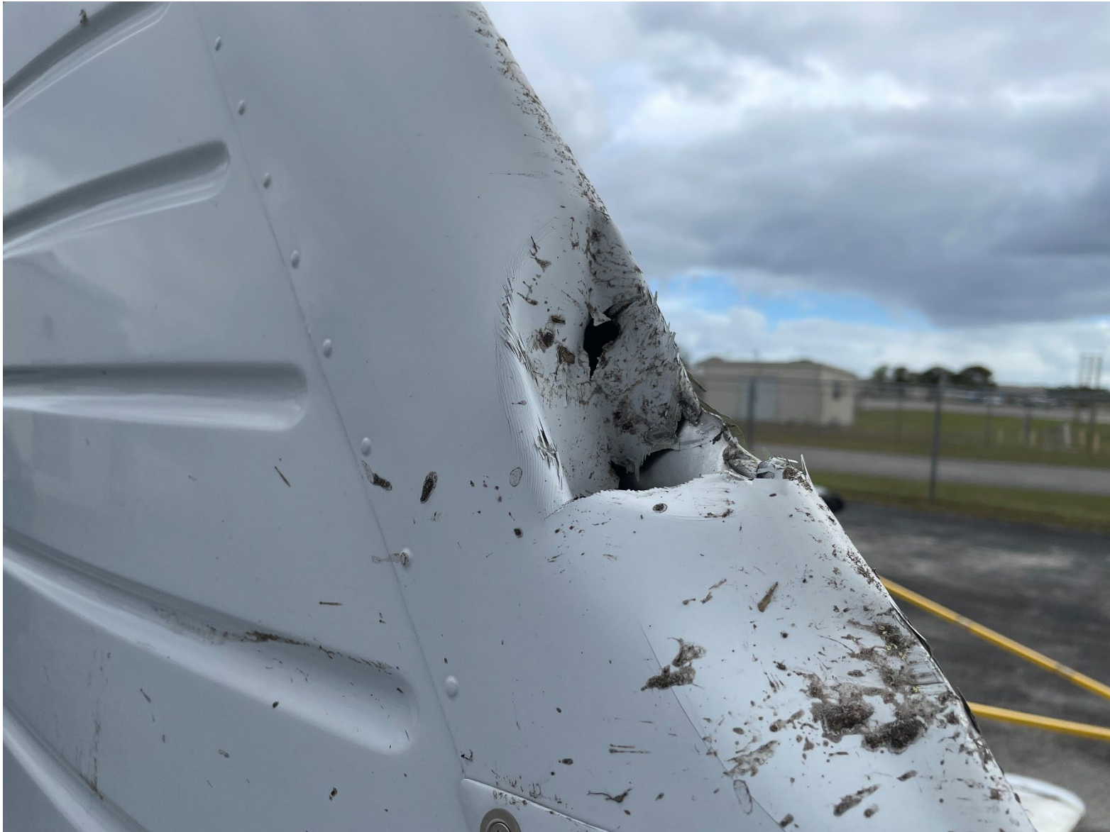
Photograph 5 - Damage to the vertical stabilizer (Courtesy of FAA)
