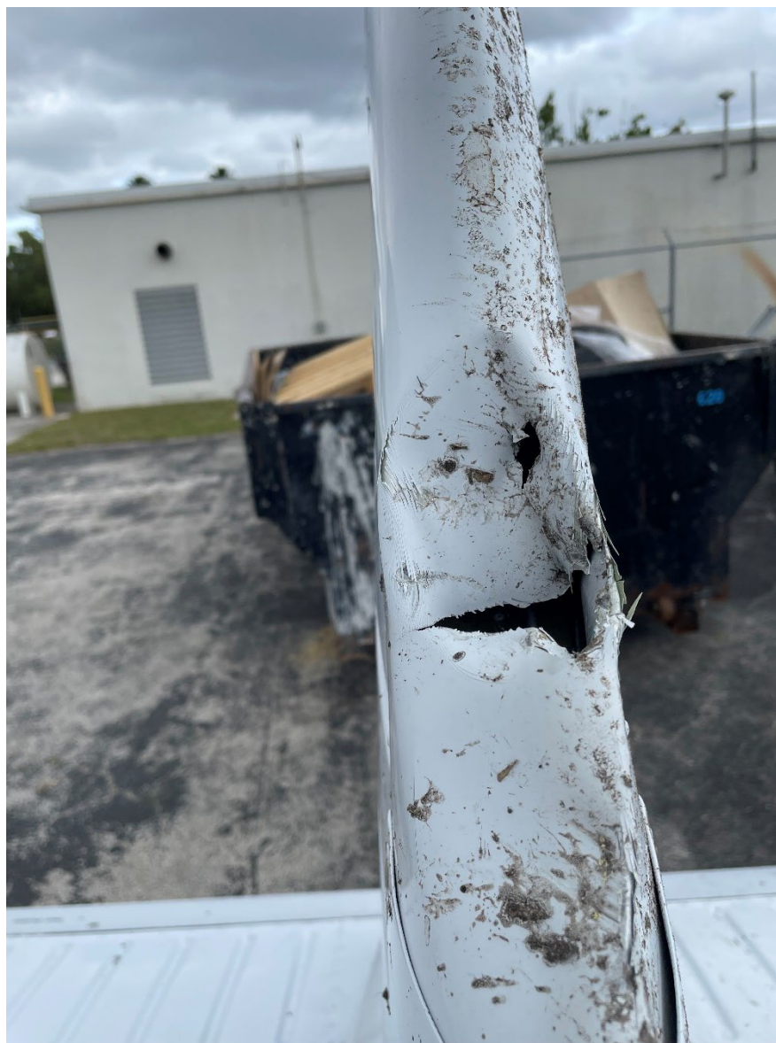
Photograph 4 - Damage to the vertical stabilizer (Courtesy of FAA)
