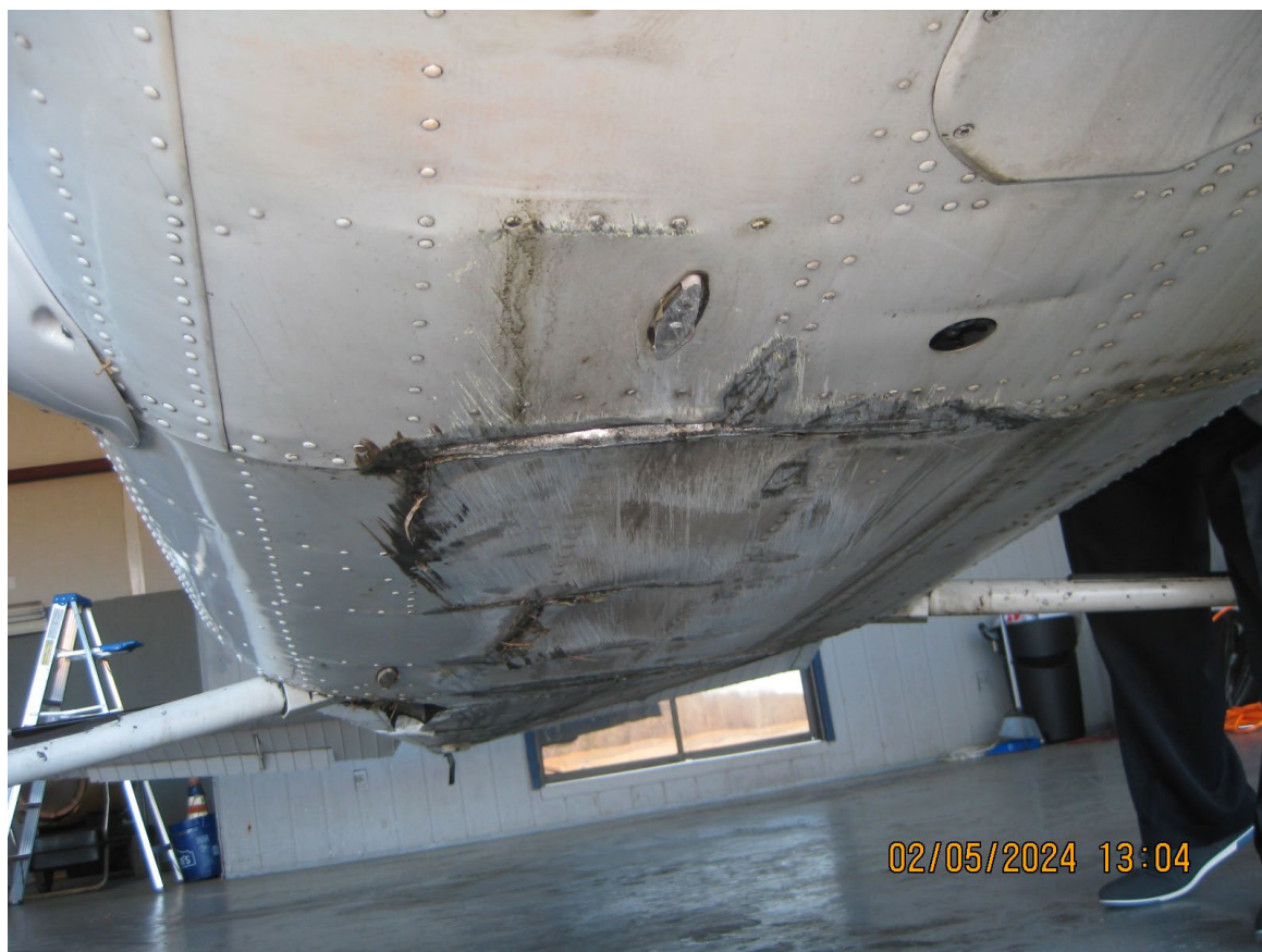
Photograph 2 - View of lower fuselage damage. (Courtesy of FAA)
