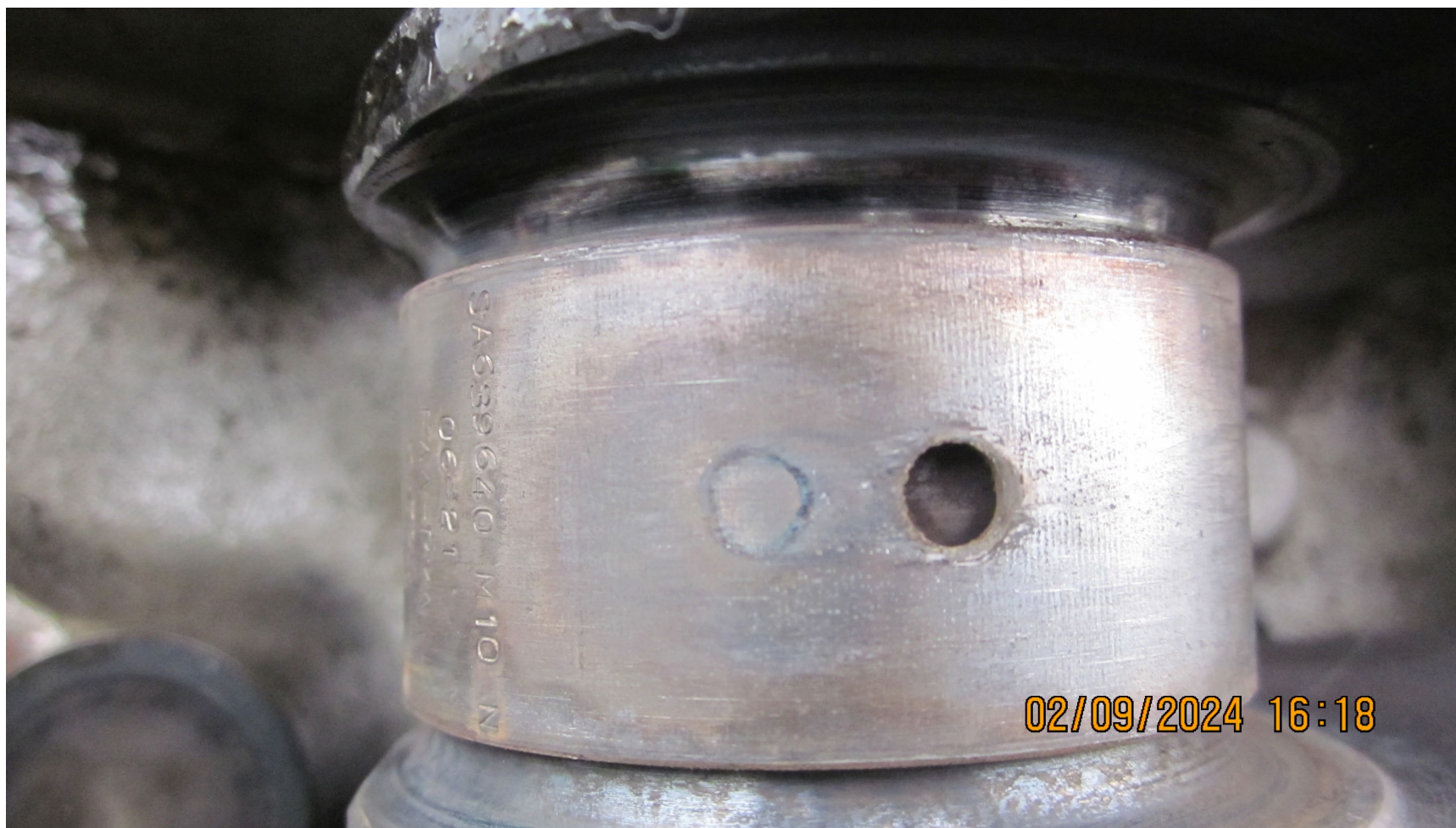
Photograph 7 - Bearing Note: alignment hole with Rod slippage.
