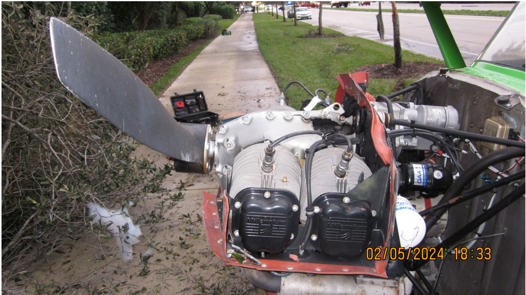
Photograph 3 - Engine Note: hole in case half (Courtesy of FAA)
