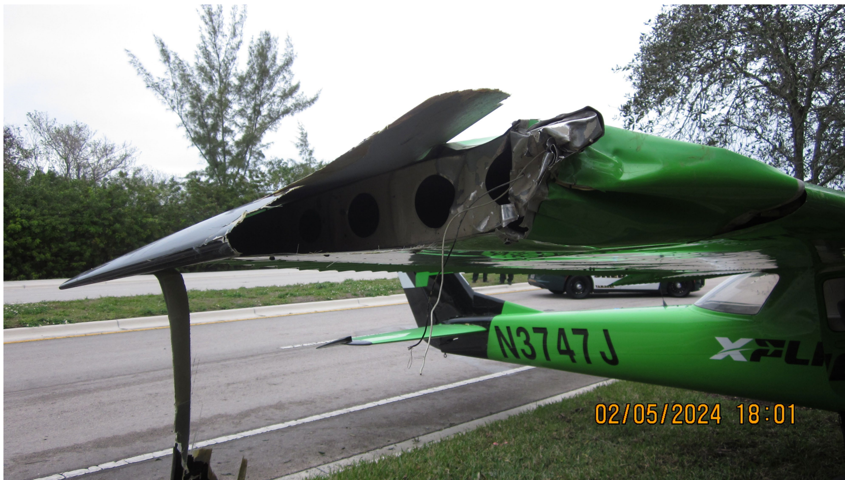
Photograph 2 - Right wing damage (Courtesy of FAA)
