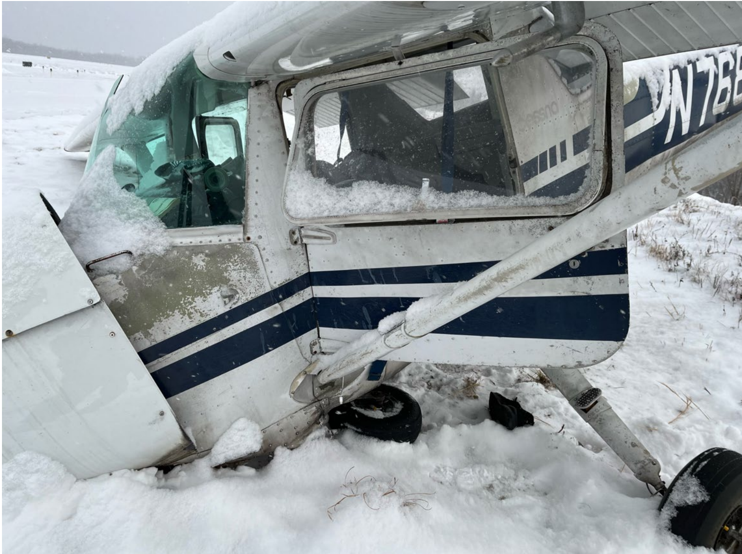
Photograph 3 - Left side of fuselage damage. Note, snow occurred post-accident. (Courtesy of FAA)
