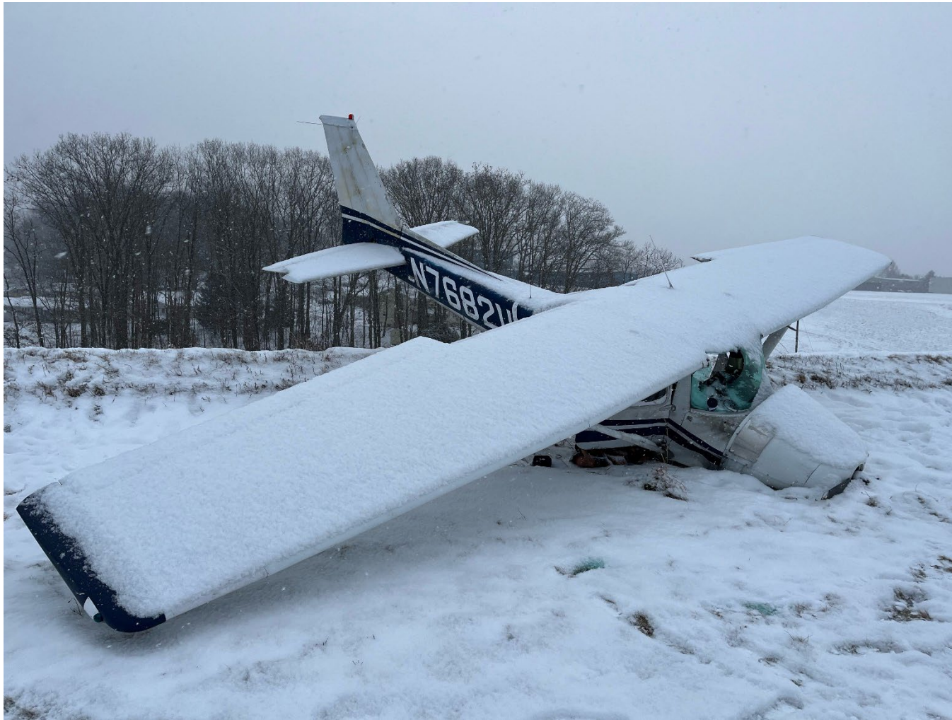
Photograph 4 - Right profile view of airplane damage. Note, snow occurred post-accident. (Courtesy of FAA)
