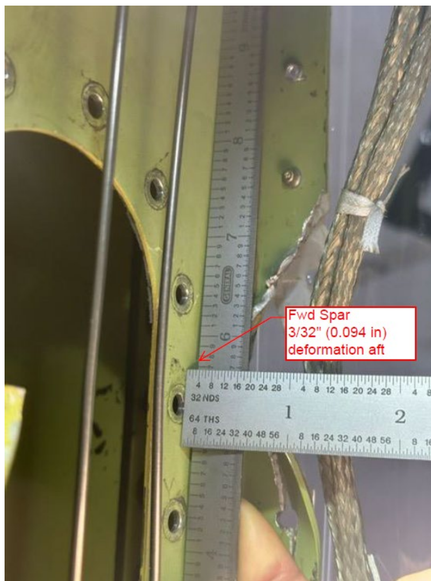
Photograph 14 - Depicting Damage to the Left Main Spar (Courtesy of Airplane Manufacturer)
