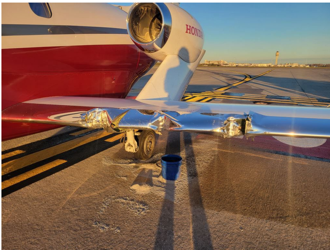
Photograph 2 - Frontal View of the Inboard Section of Left Wing, Portion of Fuselage, Left Engine. Note dents in leading edge (Courtesy of FAA)
