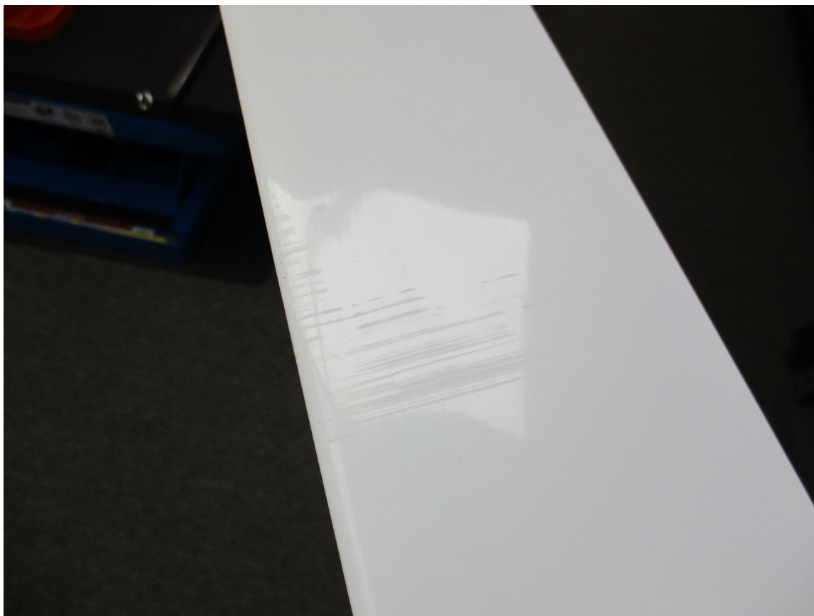
Photograph 38: Rotor blade with scuffing (Source: FAA)
