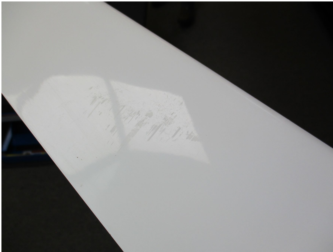
Photograph 37: Rotor blade with scuffing (Source: FAA)
