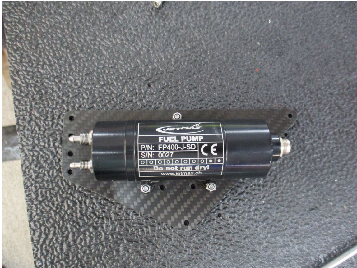
Photograph 31: Fuel pump (Source: FAA)
