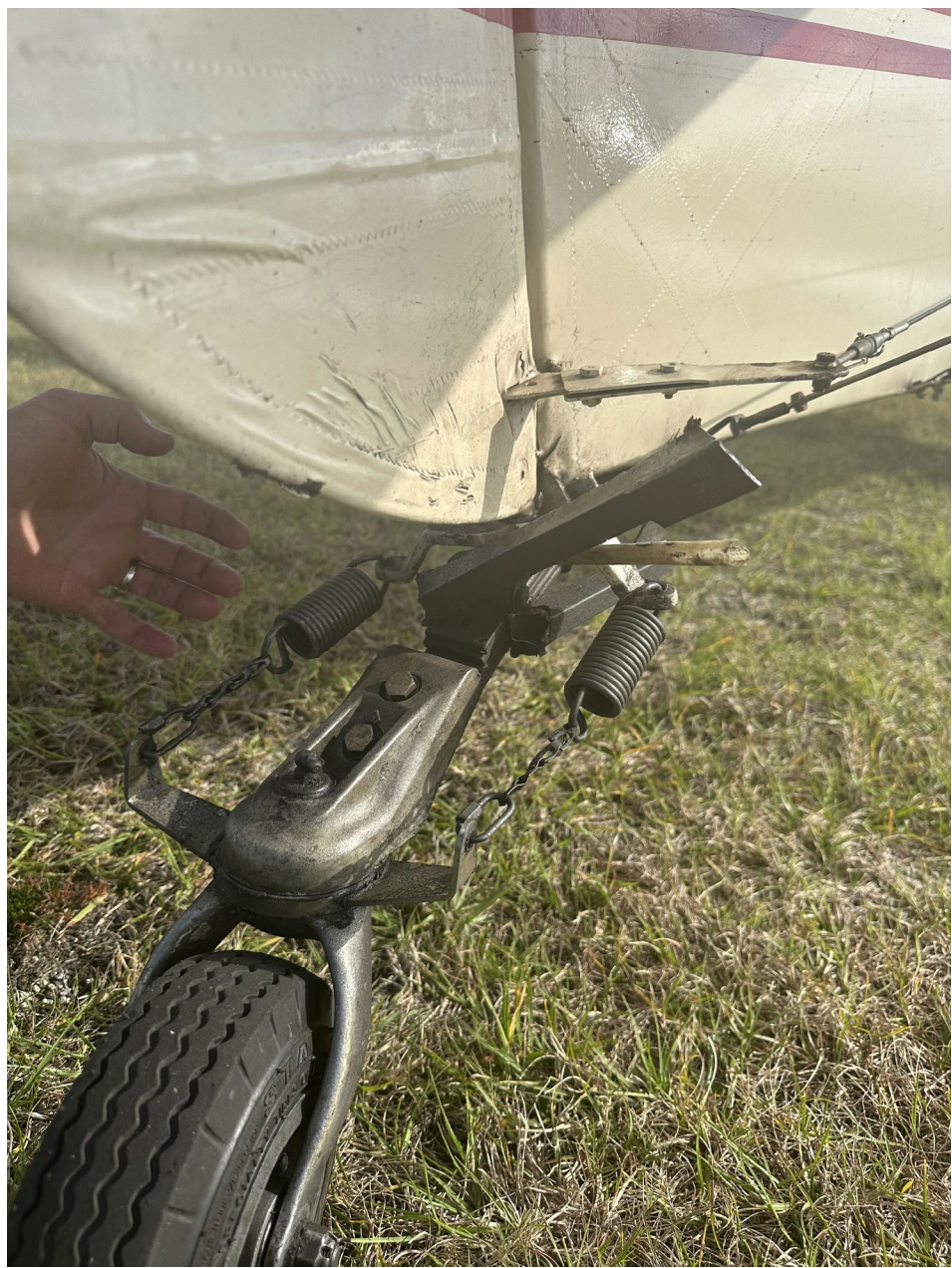
Photo 3 – View of Fractured TOST Tow Support Mount (FAA)
