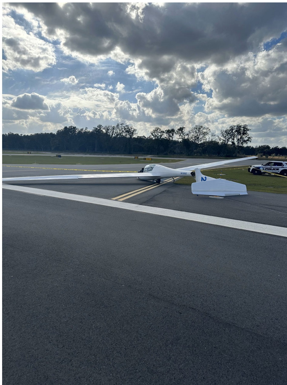
Photo 2 – View from Departure Runway of Glider’s Fractured Tail (FAA)
