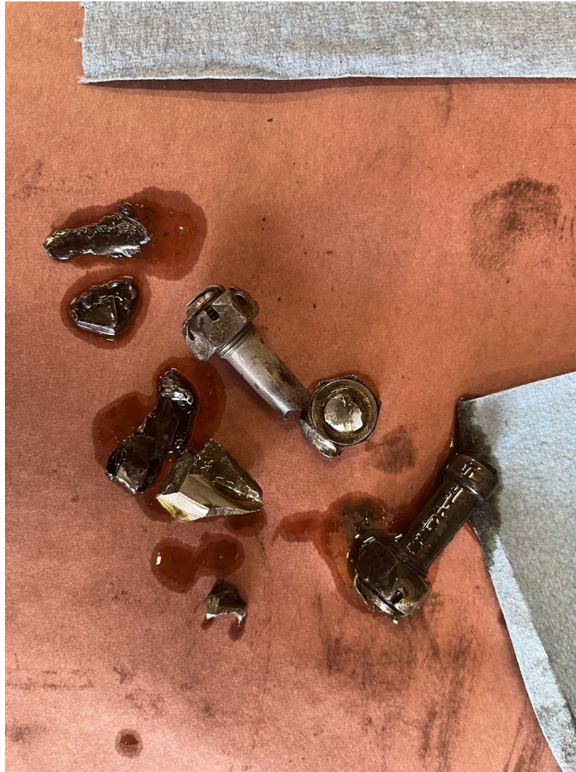
Photograph 5 - Hardware from the No. 4 connecting rod
