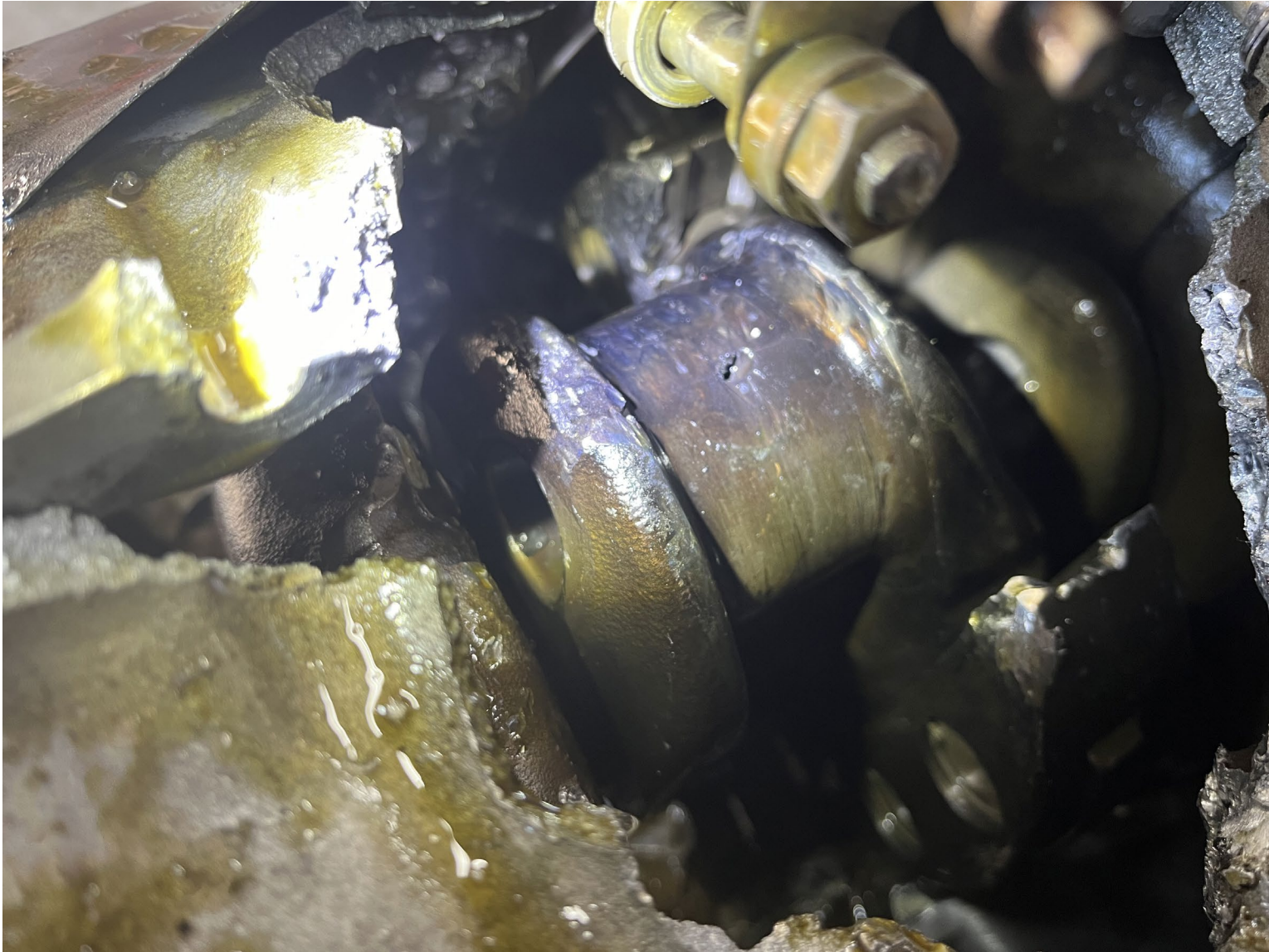
Photograph 2 - No. 4 Main journal, note: blocked oil port
