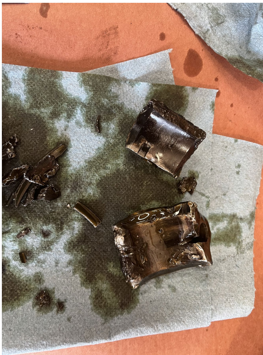
Photograph 4 - Parts of No. 4 Rod cap found in sump
