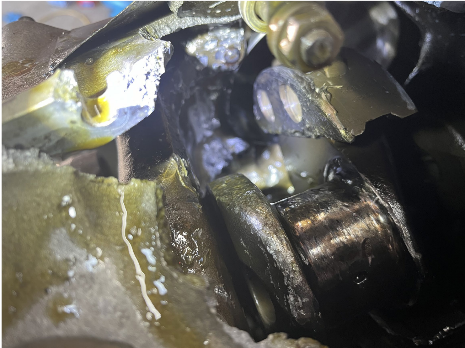
Photograph 3 - No. 4 main journal
