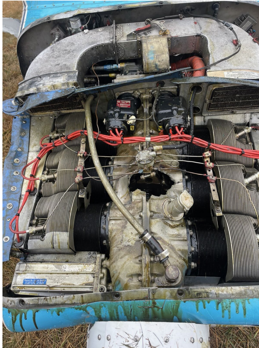
Photograph 4 - Hole in engine case (FAA)
