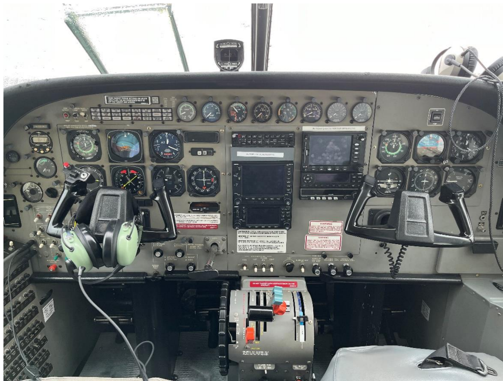
FAA On Scene Engine Controls and Inertial Separator Handle Photo
