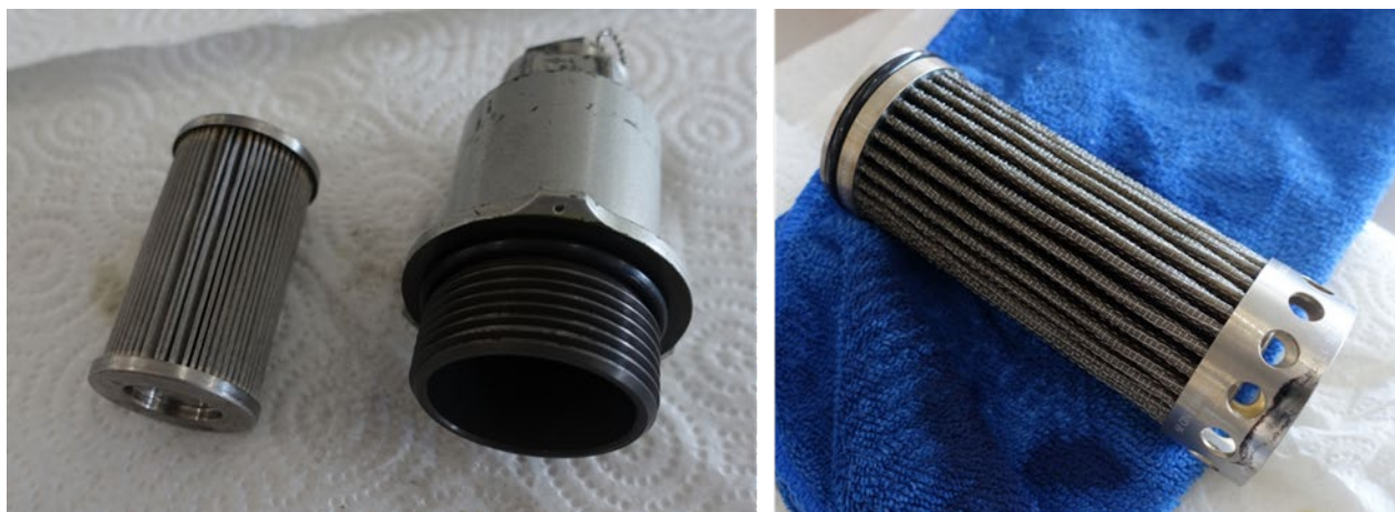
Photo 13- (L) P3 Filter, (R) Oil Filter
