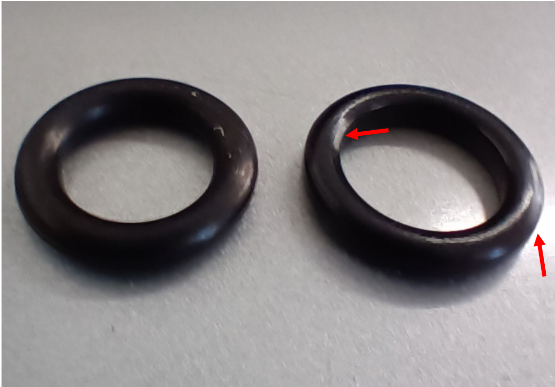
Photograph 3 – Removed o-ring and new o-ring (Courtesy of Epic Flight Academy)
