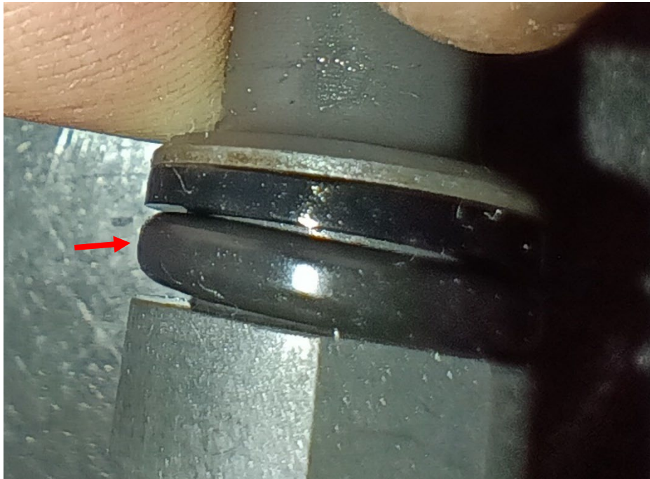
Photograph 1 – Flat spot/setting of o-ring (Courtesy of FAA)
