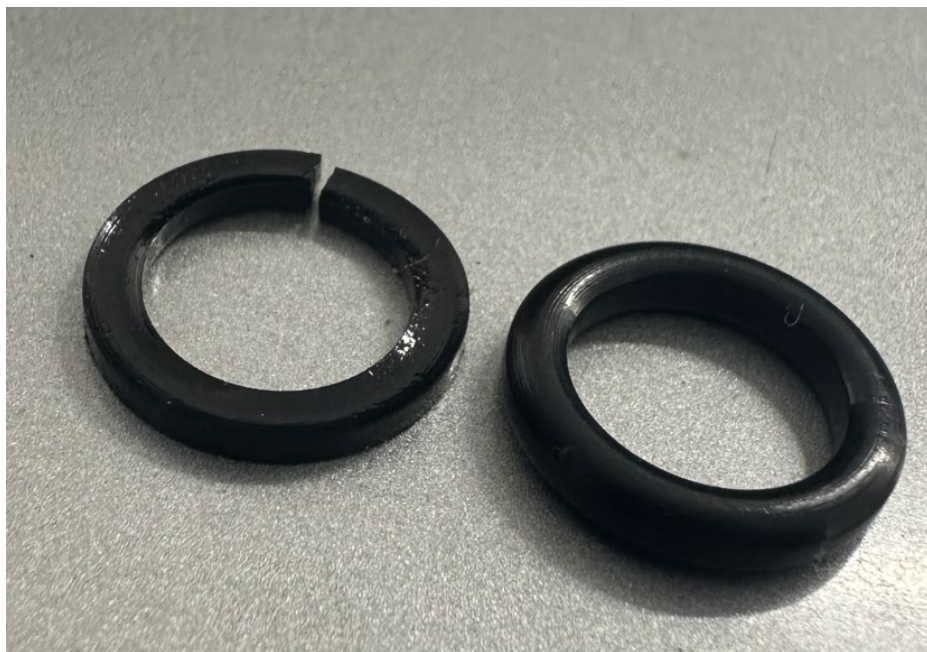
Photograph 2 – O-ring and backup removed (Courtesy of FAA)
