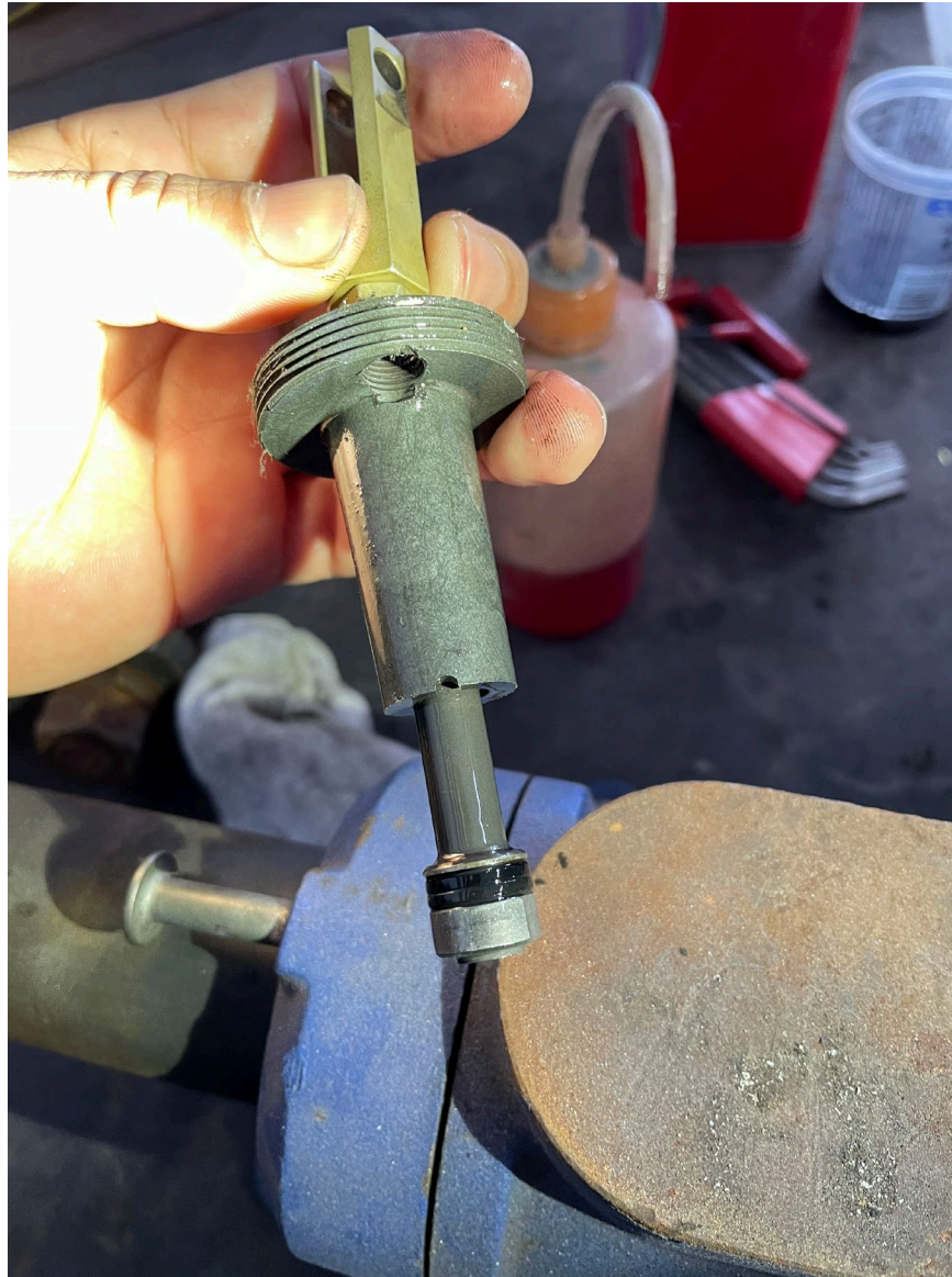
Photograph 2 - Master Cylinder Piston as Removed (Courtesy of FAA)
