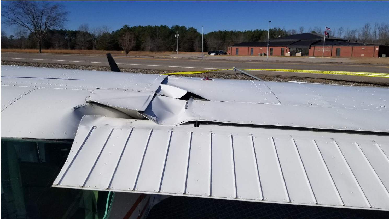
Photograph 3 - View of damaged right wing aft. (Courtesy of FAA)
