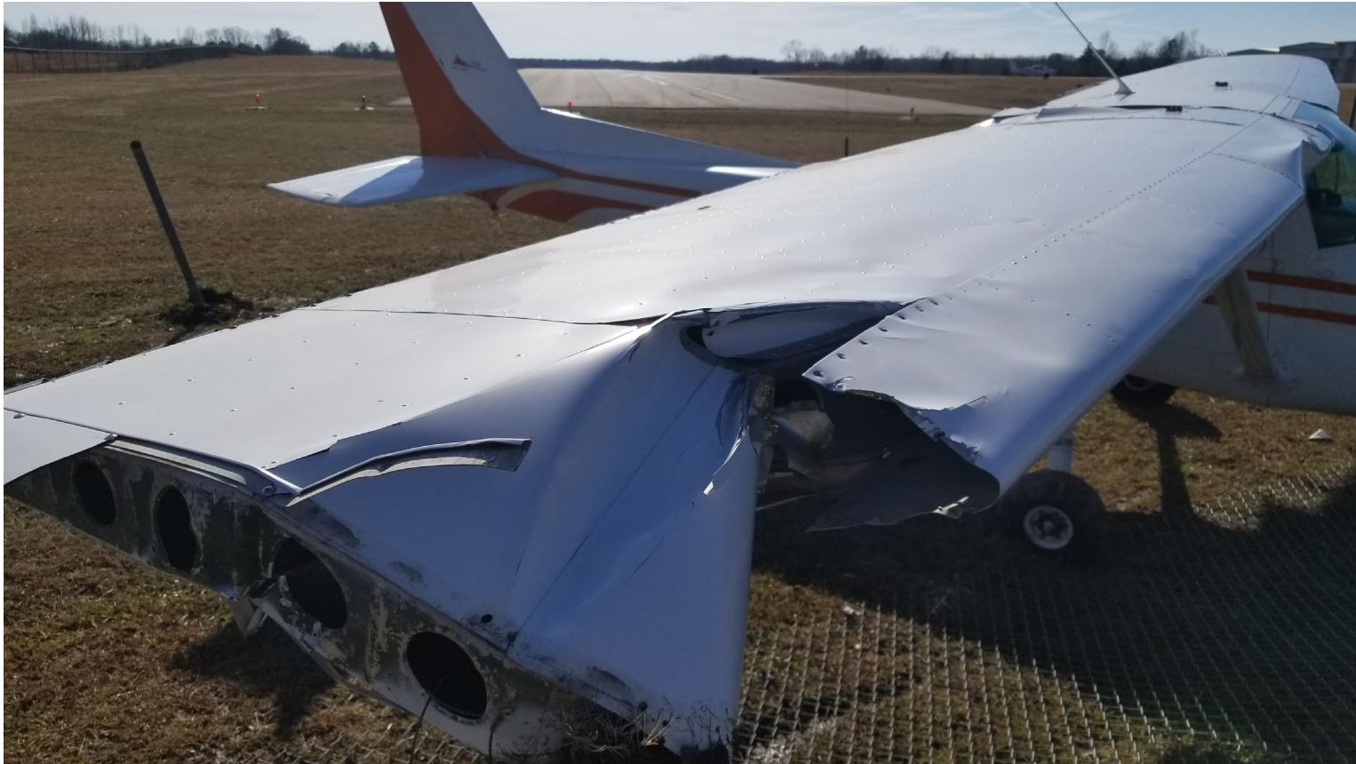
Photograph 1 - View of right damaged wing and spar. (Courtesy of FAA)
