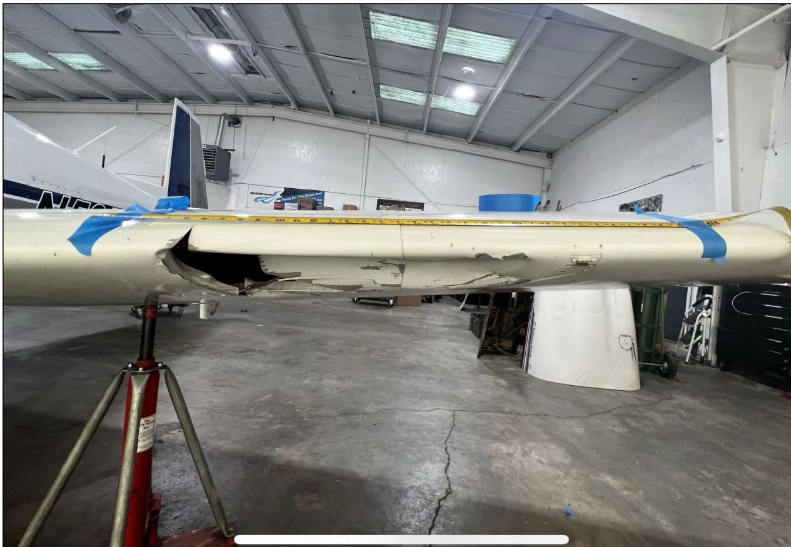
Photo 5: View of the damaged left wing (Photo Courtesy of FAA)
