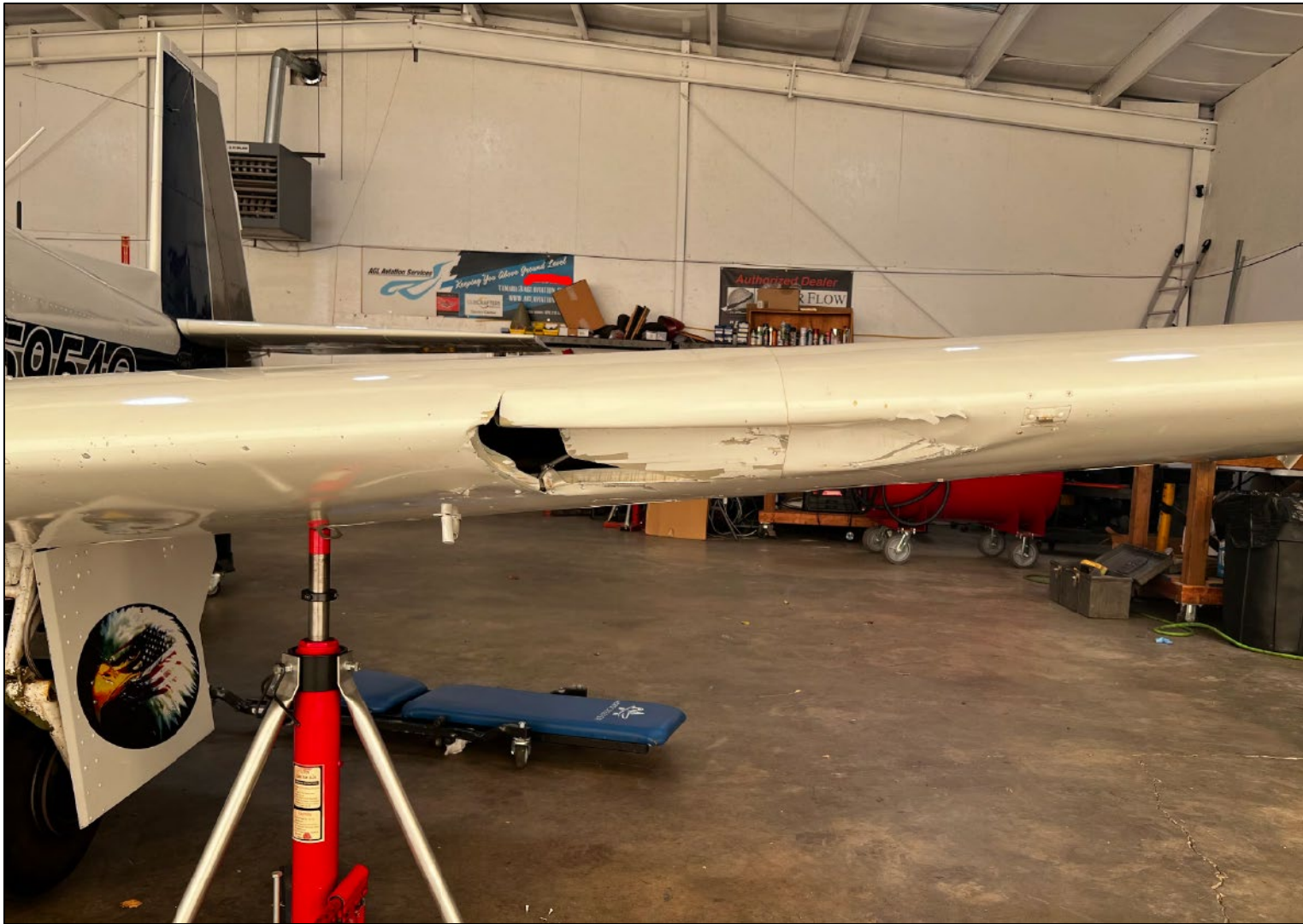
Photo 3: View of the damaged left wing (Photo Courtesy of FAA)
