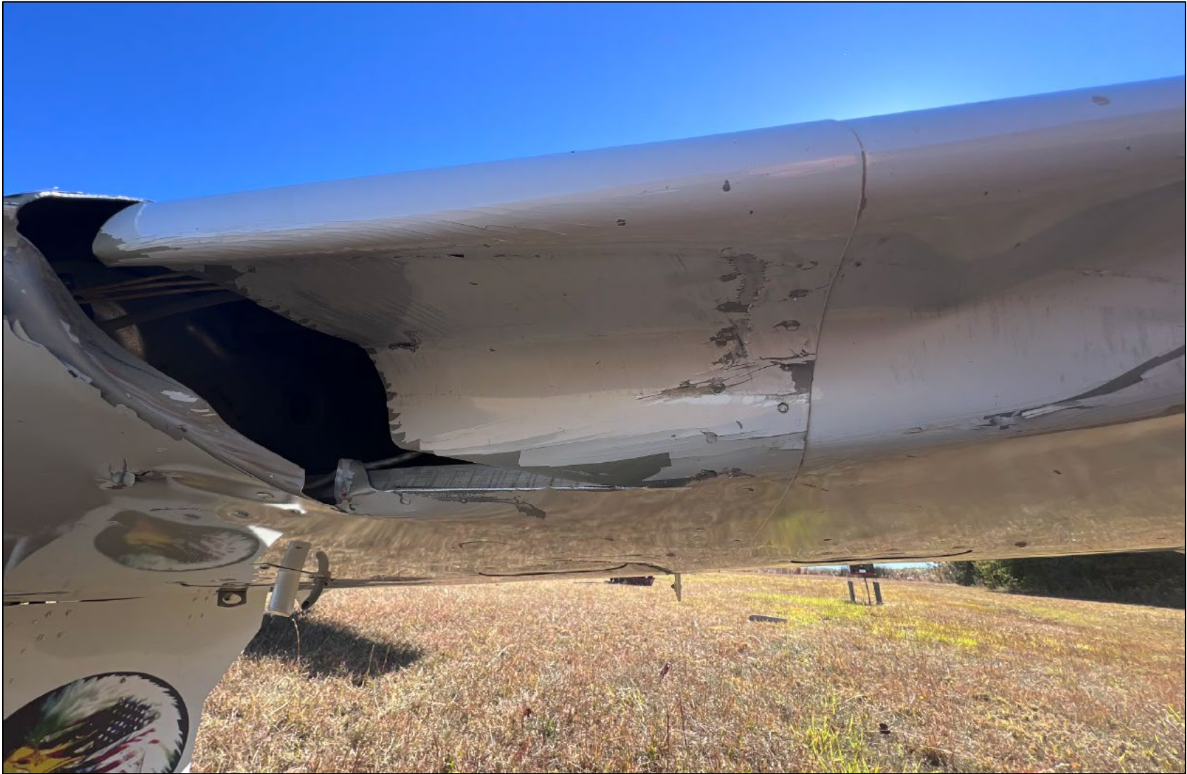
Photo 2: View of the damaged left wing (Photo Courtesy of FAA)
