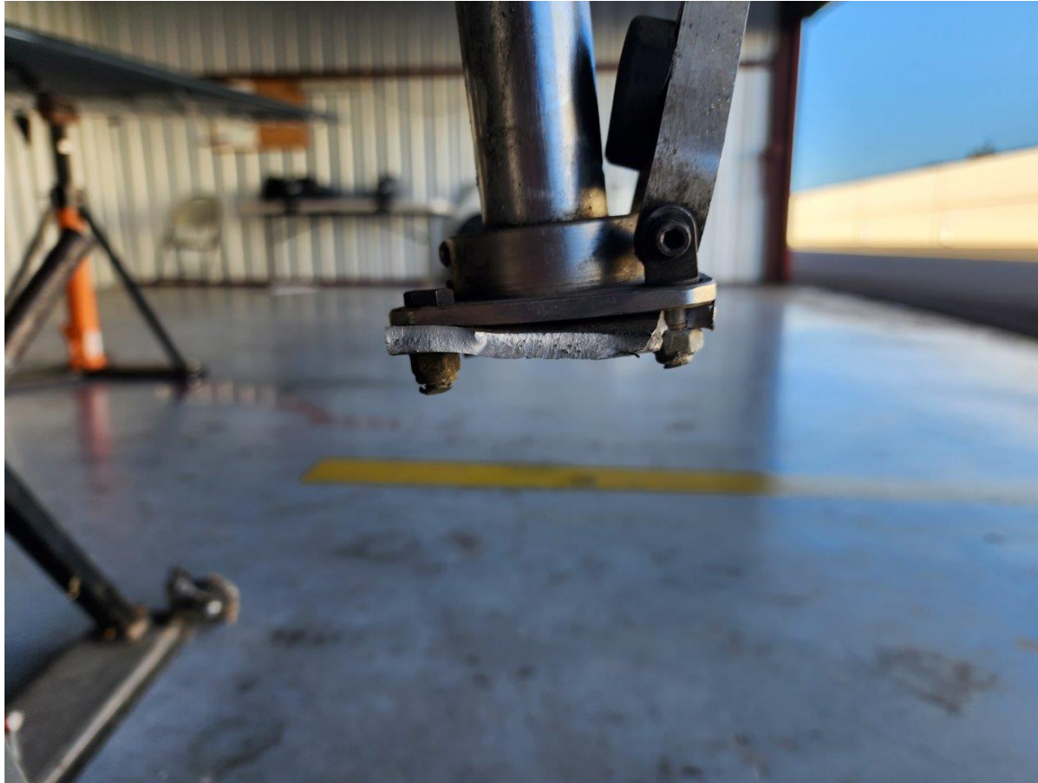
Photograph 5 - Nose wheel attach bracket (Courtesy of pilot)
