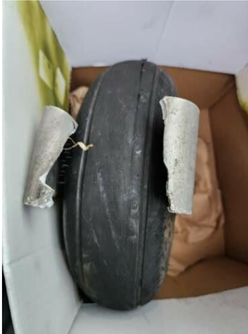
Photograph 6 - Nose wheel and attach bracket found at XSA (Courtesy of pilot)
