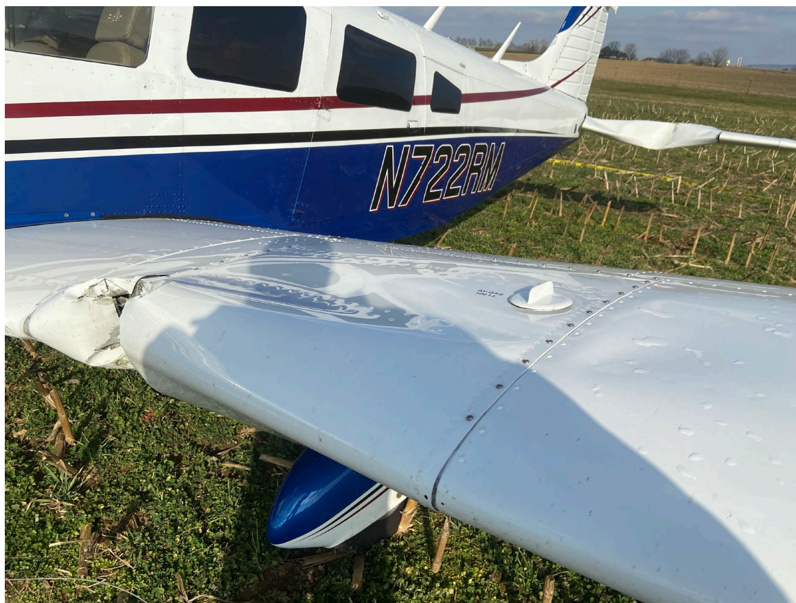
Photograph 6 - FAA Digital Photograph. View of the Inboard Portion of the Left Wing, and Left Side of the Fuselage. Note the Impact Damage on the Inboard Portion of the Main Fuel Tank.
