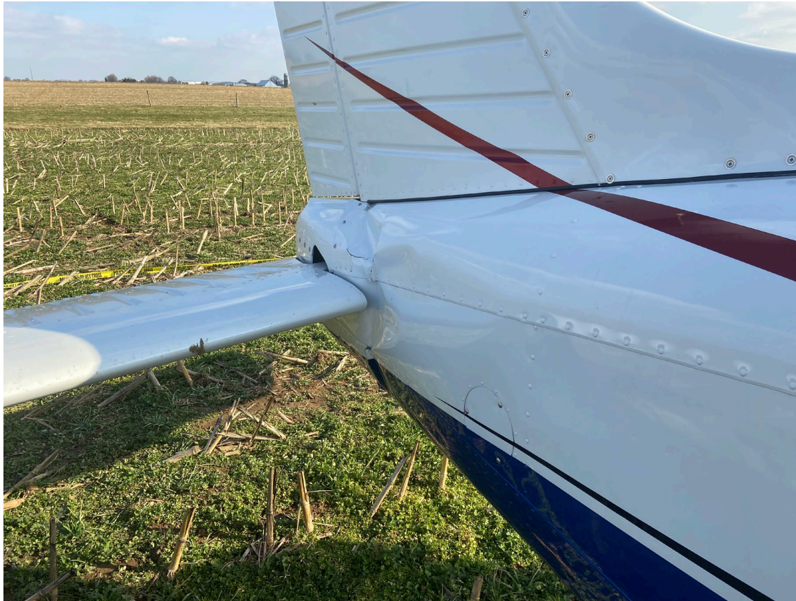
Photograph 3 - FAA Digital Photograph. Right View of Aft Empennage Showing Structural Damage Near Right Horizontal Stabilator.
