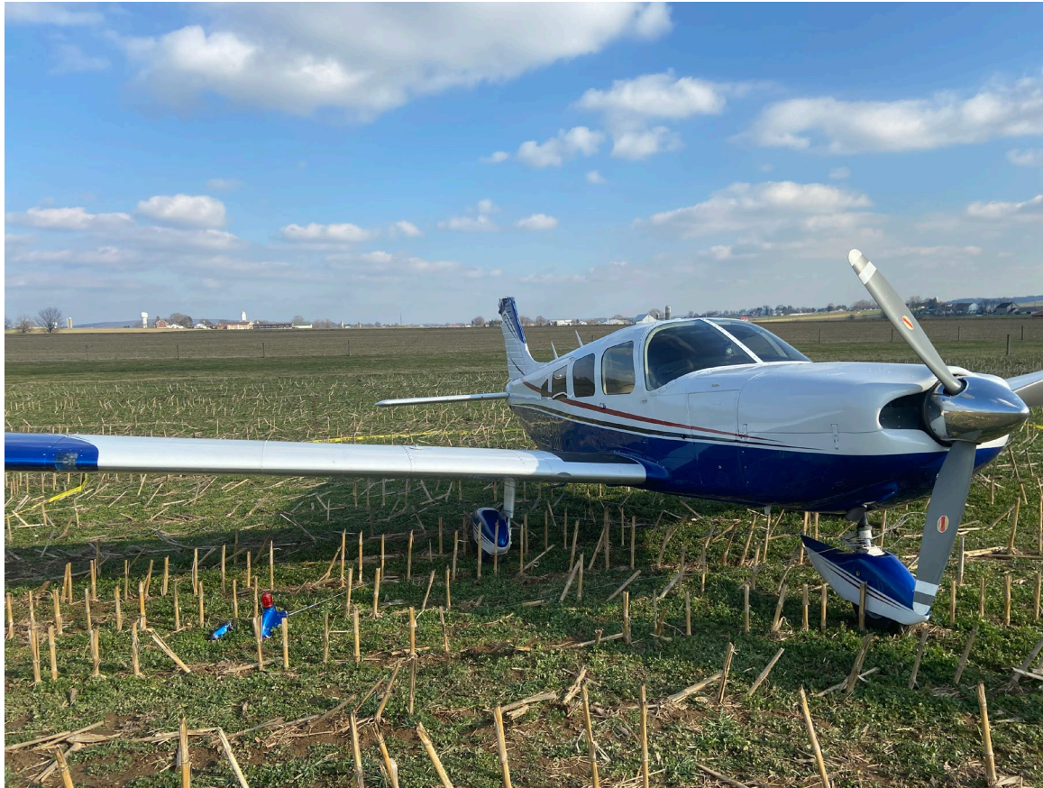
Photograph 2 - FAA Digital Photograph. Right Forward Quartering View of the Airplane at the Accident Site. Note the Lack of Damage to 2 Visible Propeller Blades.
