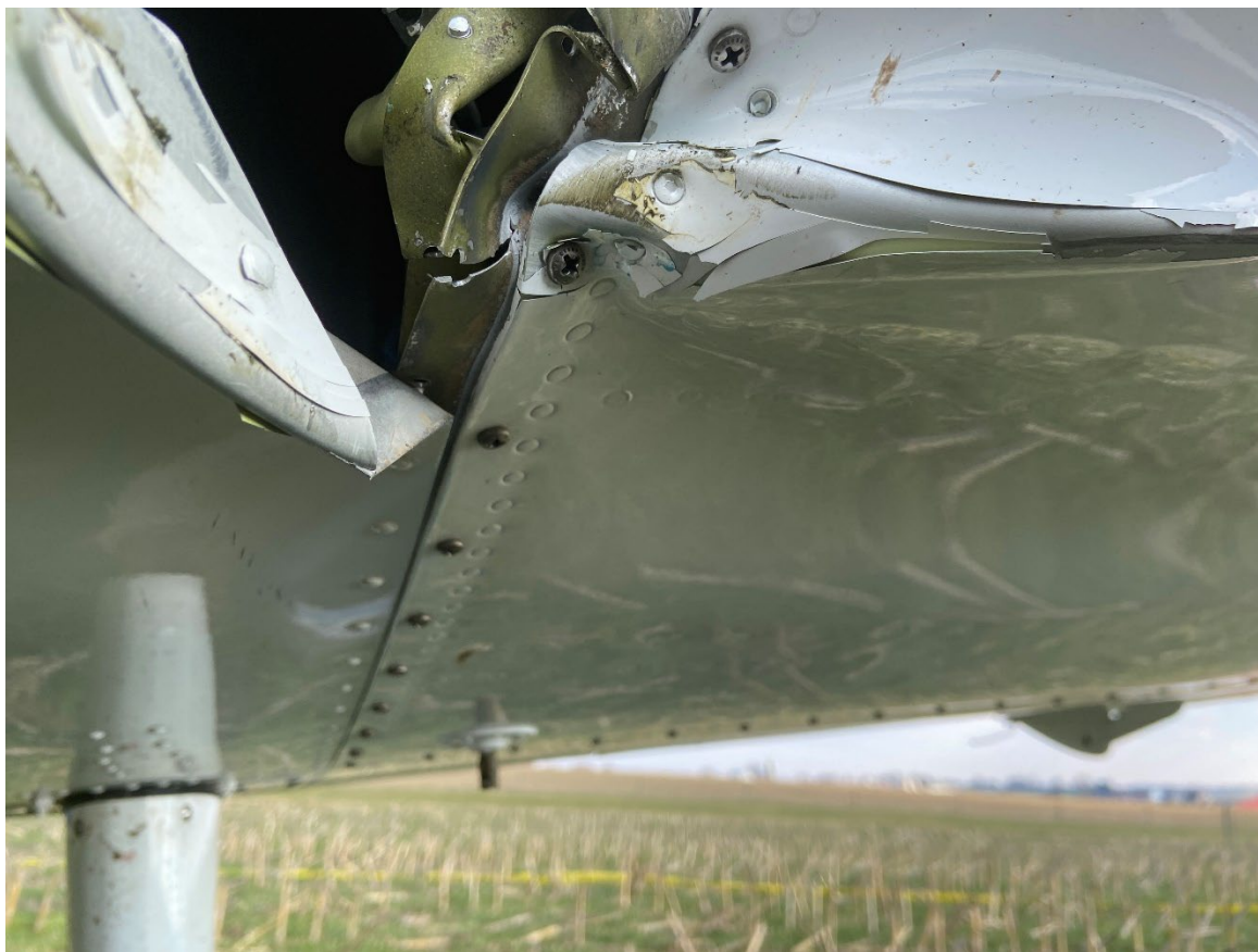
Photograph 8 - FAA Digital Photograph. View of the Lower Wing Skin of the Left Wing Adjacent to the Impact Damage to the Fuel Tank. Note the Absence of Fuel Stains.
