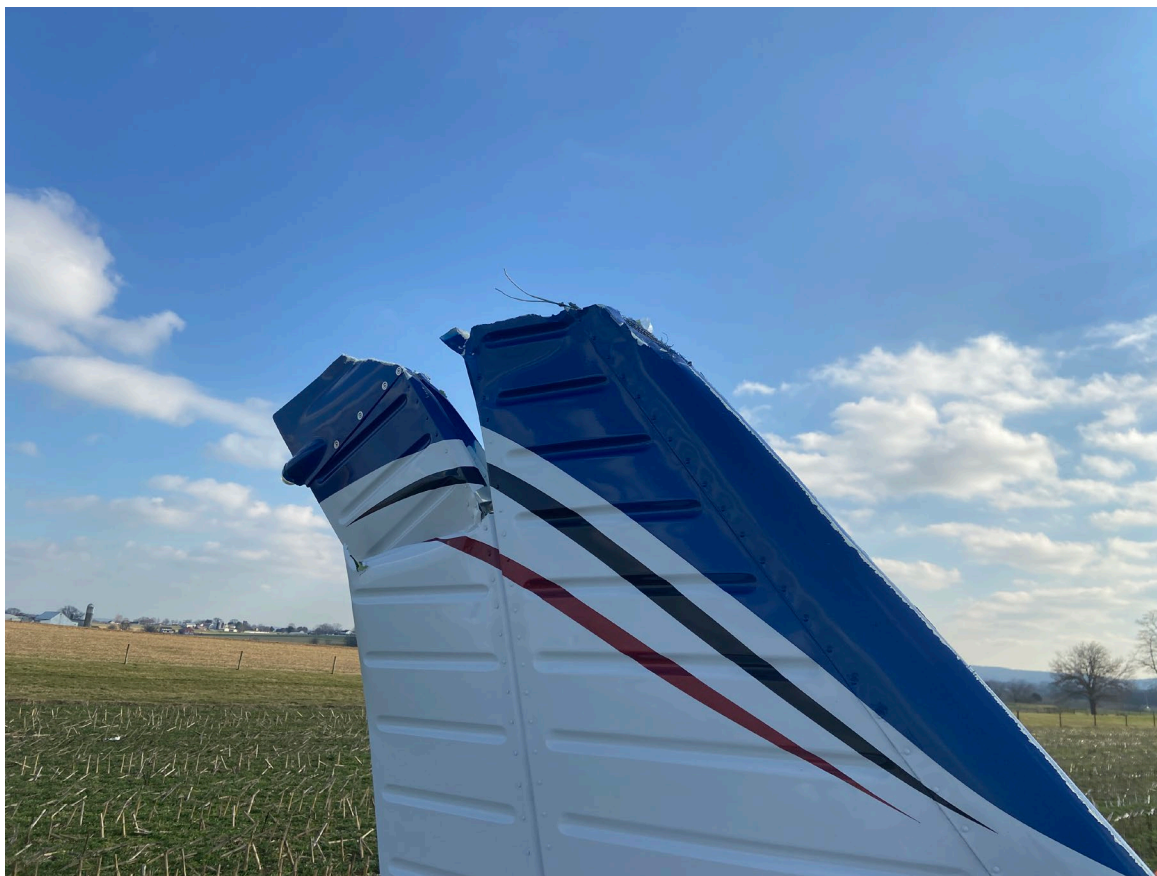
Photograph 4 - FAA Digital Photograph. Right Side View of the Upper Portion of the Vertical Stabilizer and Rudder. Note the Damage to the Spar of the Rudder.
