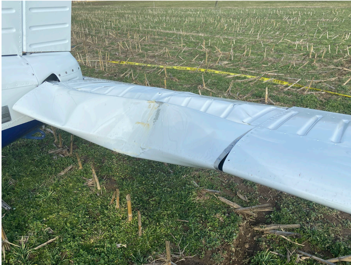
Photograph 5 - FAA Digital Photograph. View of a Portion of the Left Horizontal Stabilator. Note the Extensive Structural Damage
