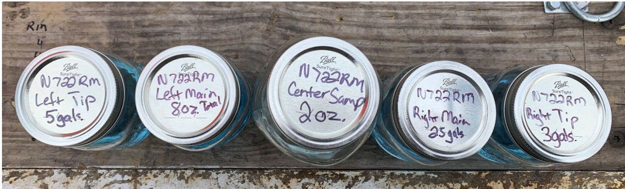
Figure 1: Digital Photograph From Anglin Air. Documents an Initial Sample of Fuel and/or the Complete Amount Drained From each Tank, and the Quantity Drained From Each Fuel Tank.
