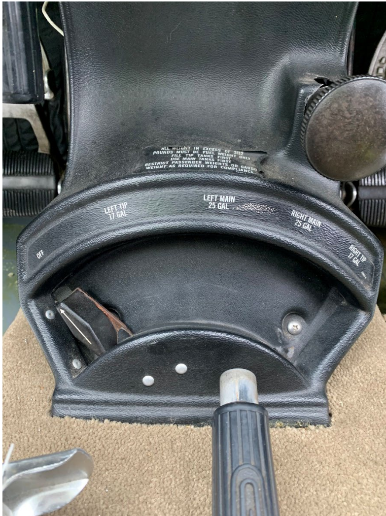
Figure 1: Digital Photograph From Anglin Air personnel. View of the Fuel Selector.
