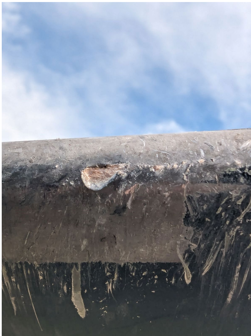
Photograph 1 - View of damage to the main rotor blade (Courtesy of FAA)
