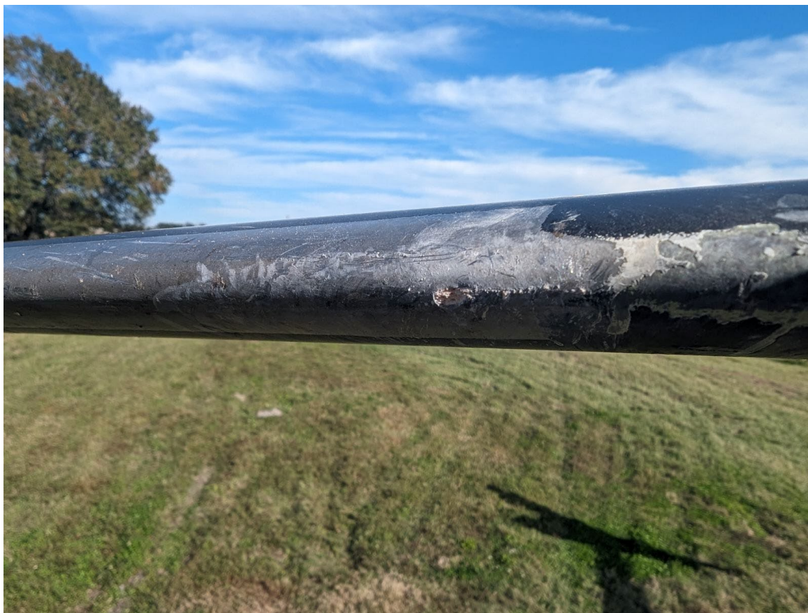
Photograph 2 - View of damage to the main rotor blade (Courtesy of FAA)
