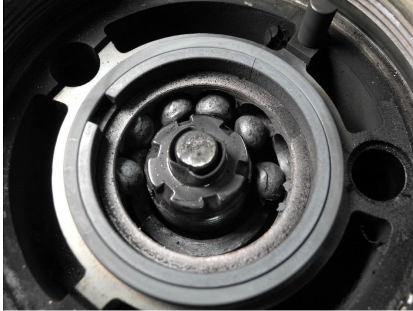
Photo 27 - No. 8 Bearing - Disintegrated
