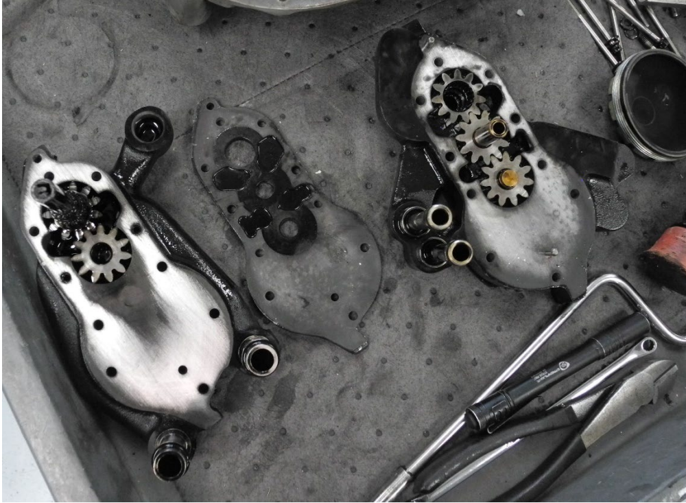
Photo 11 - Oil Pumps - Undamaged
