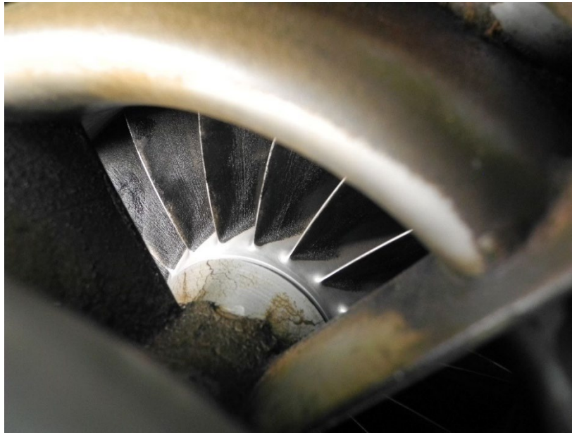
Photo 5 - Impeller Vanes Leading Edges - Undamaged
