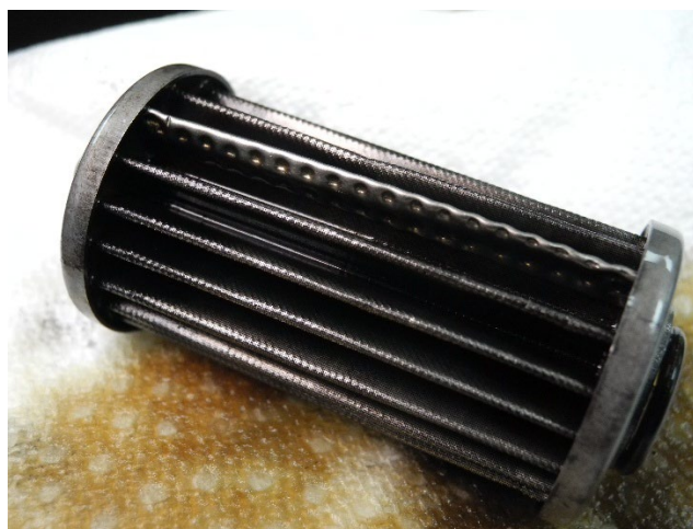
Photo 4 - Engine Oil Filter - Clean
