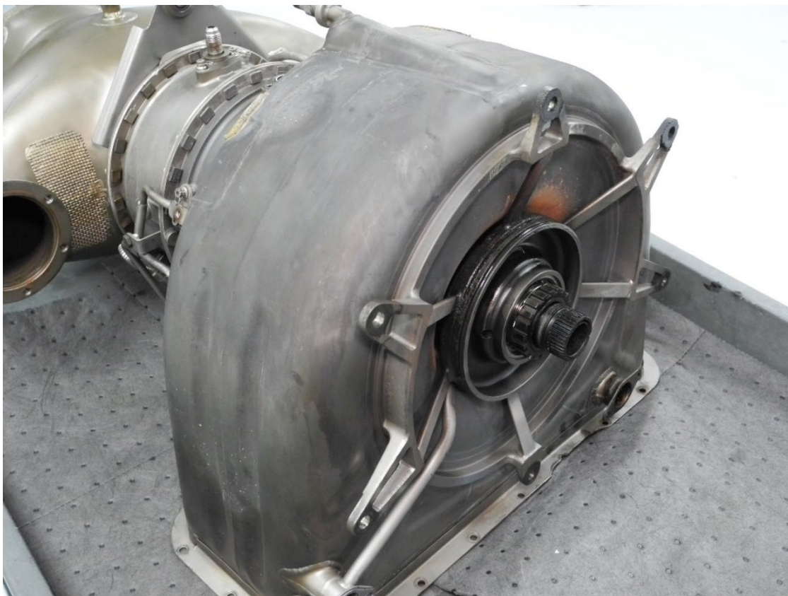
Photo 12 - Exhaust Collector Support Housing - AGB Side
