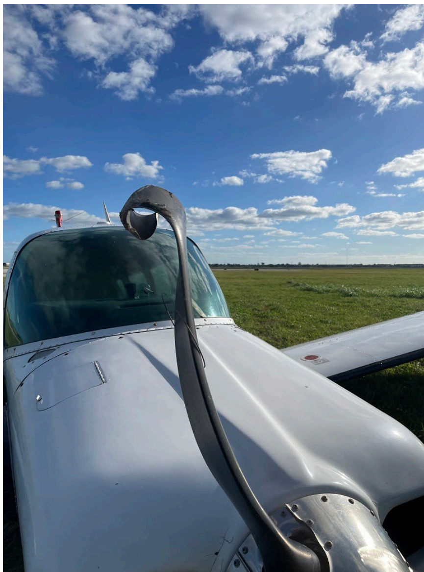
Photograph 3 - Propeller Tip Curling (Courtesy of FAA)
