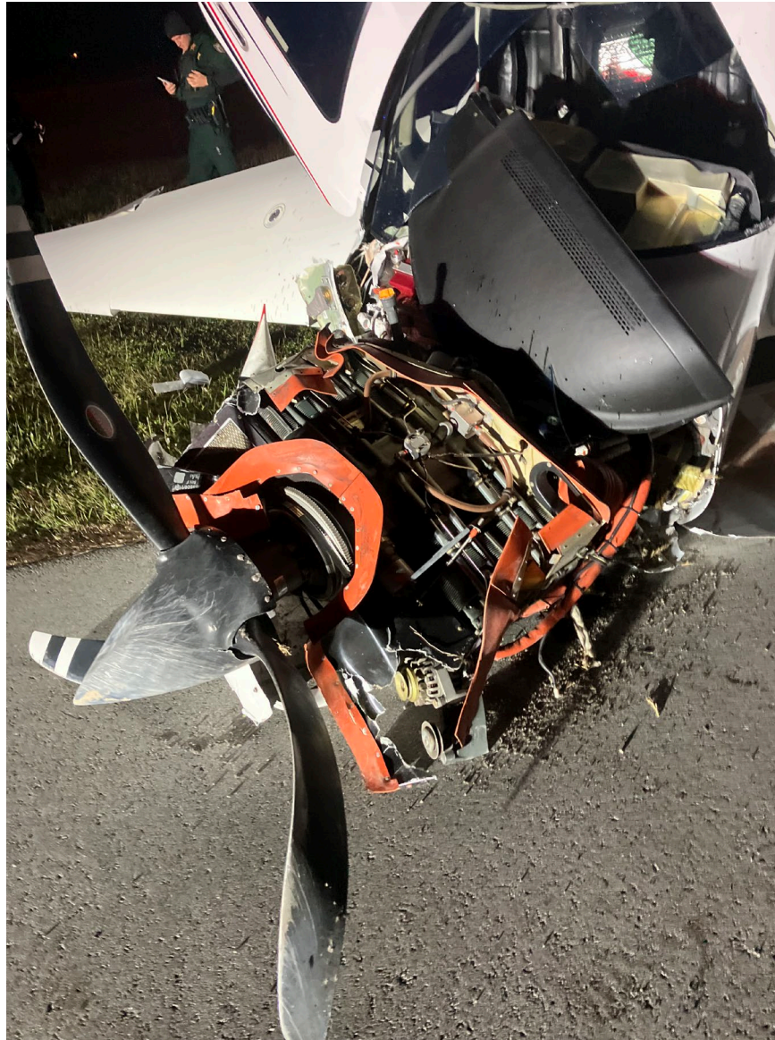
Photograph 3 - Damage to Engine and Firewall (Courtesy of FAA)
