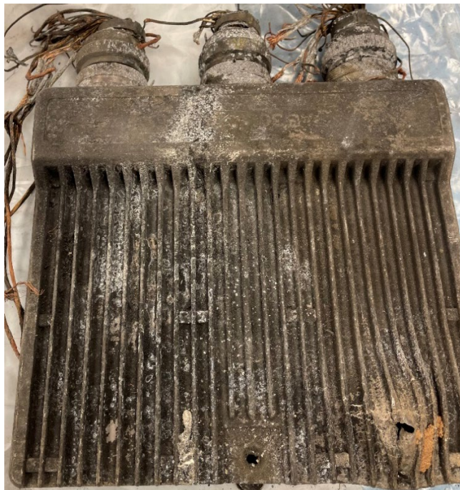
Figure 1. Austro AE300 EECU as received by the NTSB Vehicle Recorder Laboratory.
