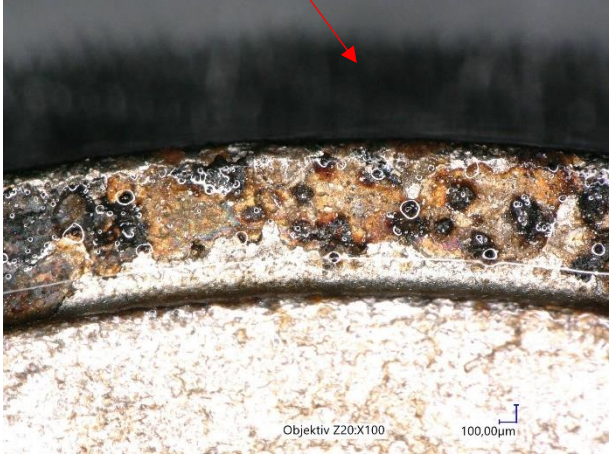
Figure 55 - Injector 2, armature guide x50
