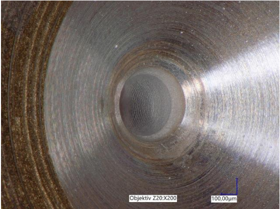
Figure 58 - Injector 3, A-throttle ~35° left
