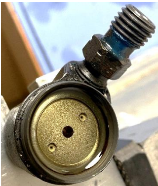
Figure 38 - Injector 4, armature removed
