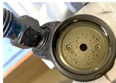
Figure 16 - Injector 3, armature removed
