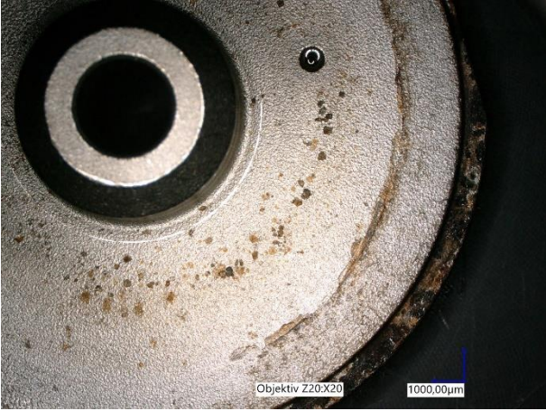
Figure 68 - Injector 4, armature guide x20 (1)
