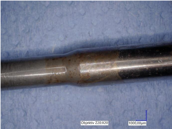
Figure 70 - Injector 4, control piston x20 (1)
