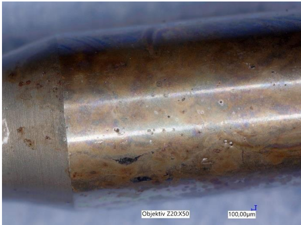
Figure 62 - Injector 3, control piston x50
