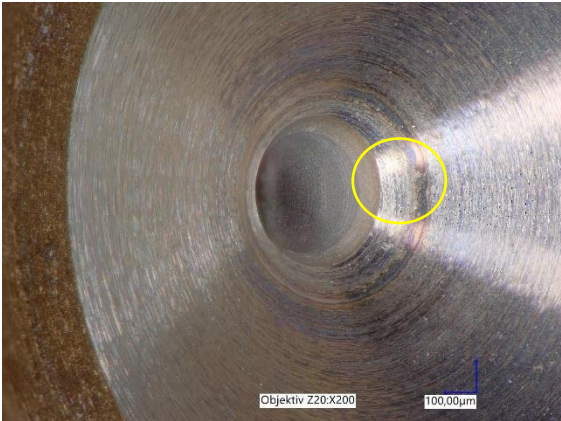
Figure 64 - Injector 4, A-throttle ~35° left
