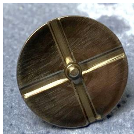
Figure 15 - Armature, top side
