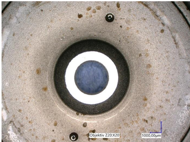
Figure 44 - Injector 1, armature guide x20
