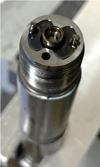
Figure 24 - Injector 3, injector nozzle removed
