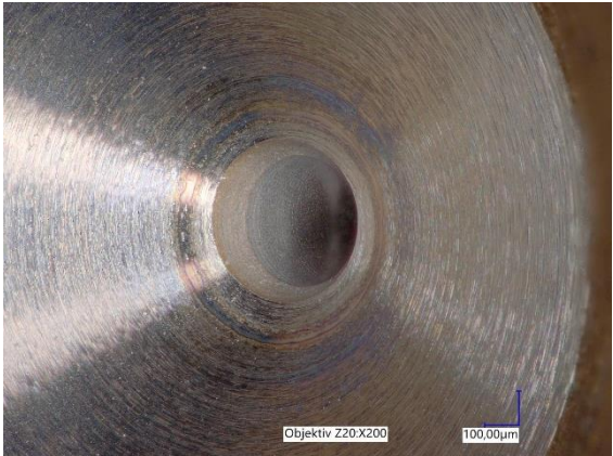
Figure 65 - Injector 4, A-throttle ~35° right
