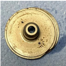
Figure 29 - Armature guide injector 1, bottom side
