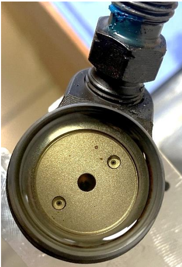
Figure 34 - Injector 2, armature removed
