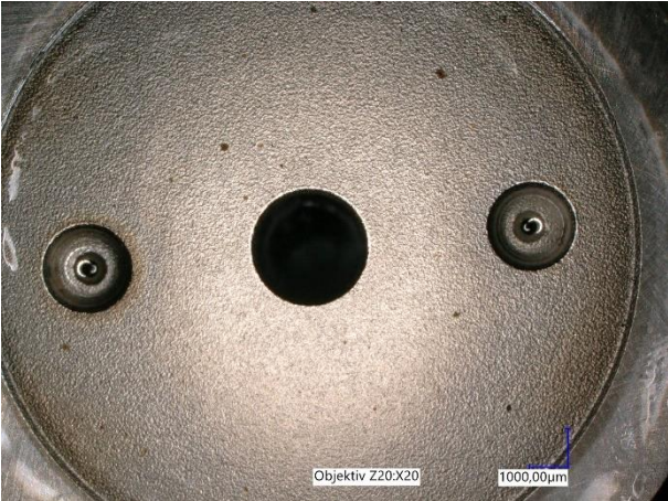
Figure 66 - Injector 4, armature guide top side x20
