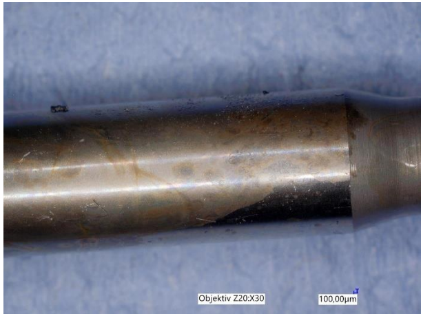
Figure 48 - Injector 1, corrosion on control piston
