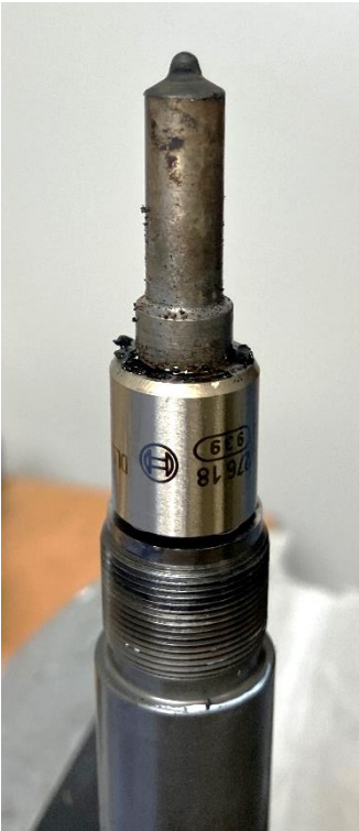
Figure 21 - Nut to secure the injector nozzle removed
