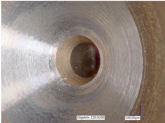
Figure 51 - Injector 2, A-throttle ~35° right
