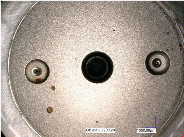
Figure 52 - Injector 2, armature guide top side x20
