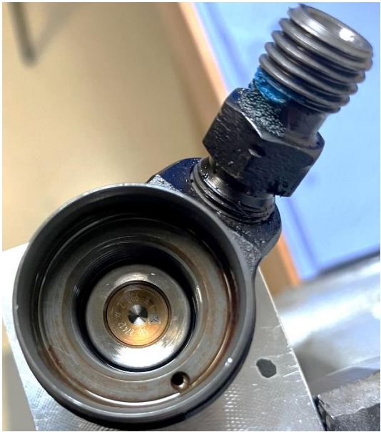
Figure 31 - Injector 1, armature guide removed
