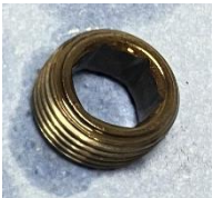
Figure 23 - Screw with secures the A-throttle
