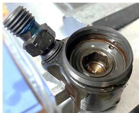
Figure 19 - Injector 3, armature guide removed
