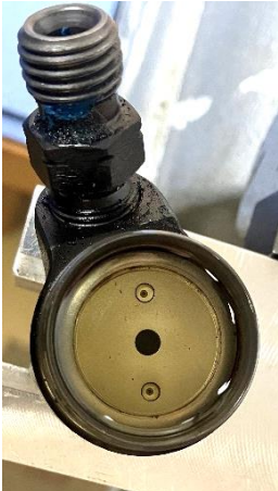
Figure 30 - Injector 1, armature removed
