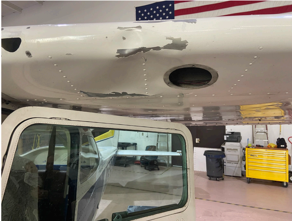
Photograph 1 - Impact Damage to Left Wing (Courtesy of FAA)
