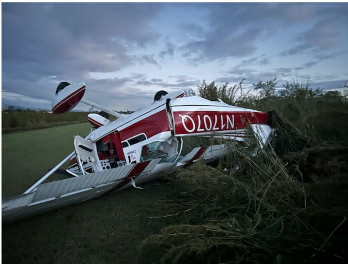
Photograph 1 -Right Side Tail Structure Damage (Courtesy of FAA)
