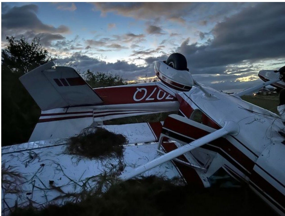
Photograph 2 - Left Side Tail Structure Damage (Courtesy of FAA)
