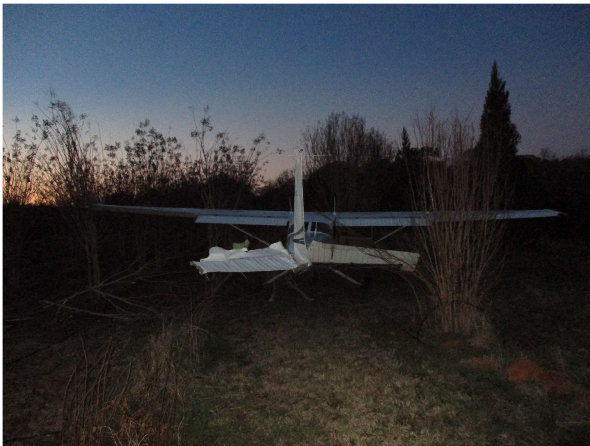
Photograph 1 - Rear view of airplane showing both rear horizontal stabilizers damaged. (Courtesy of FAA)
