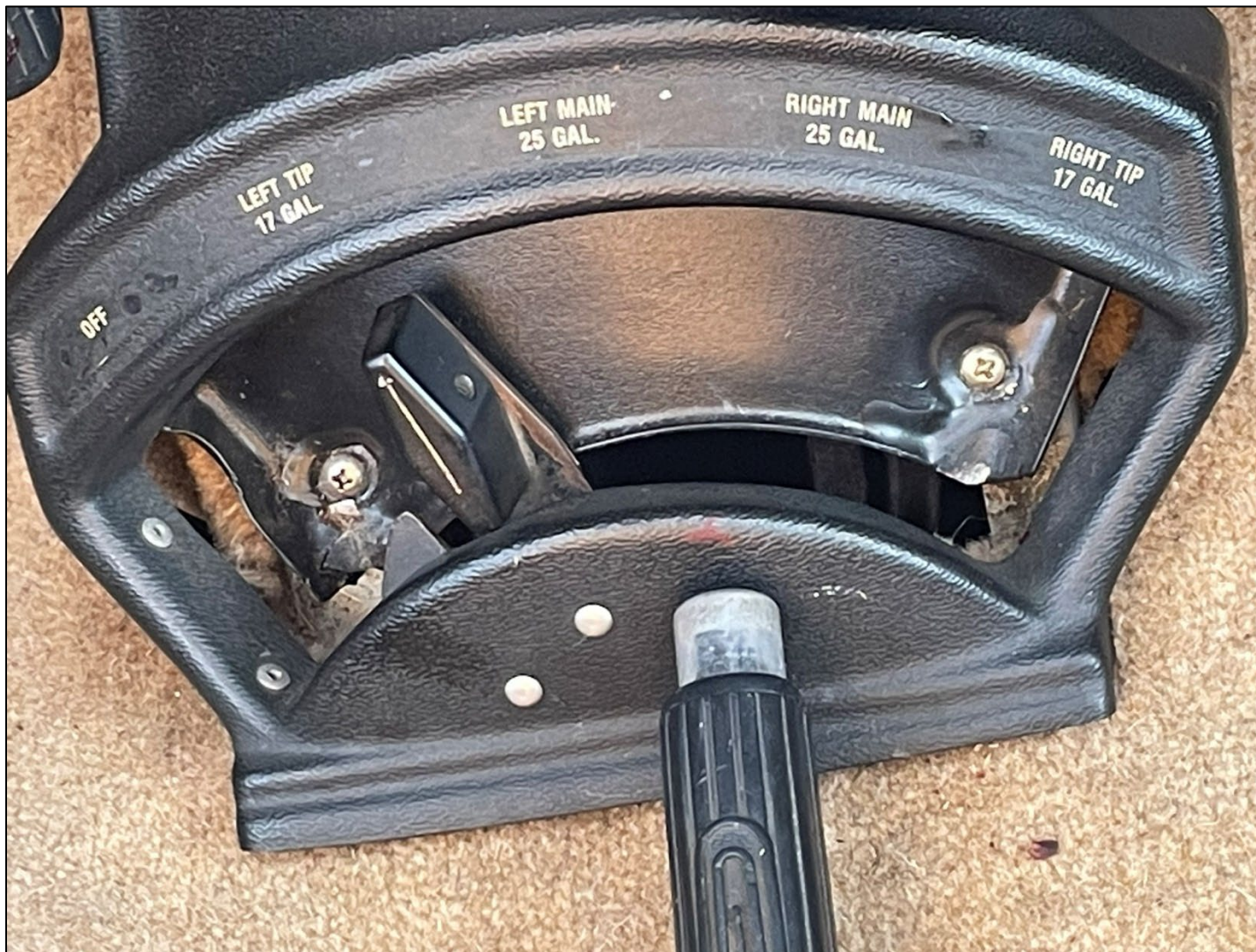
Photo 2: View of the fuel selector as observed at the accident site (Selected, Left Tip) (Photo Courtesy FAA)
