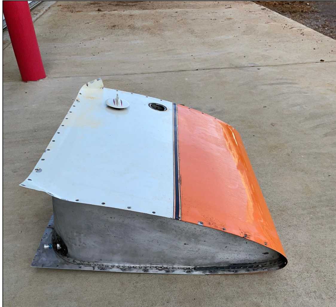
Photo 5: View of the left main tank separated from the wing, with no leaks observed upon filling with water.
