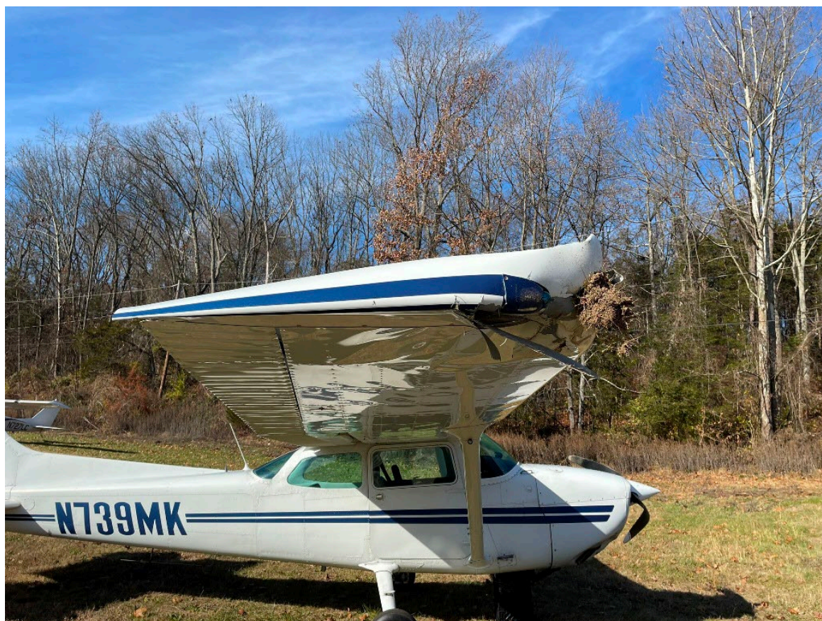
Photograph 1 - Damage to Right Wing (Courtesy of FAA)
