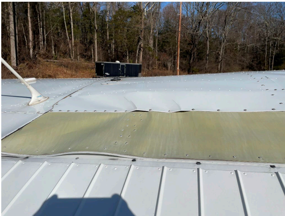
Photograph 2 - View of Damage to the Top of the Right Wing (Courtesy of FAA)
