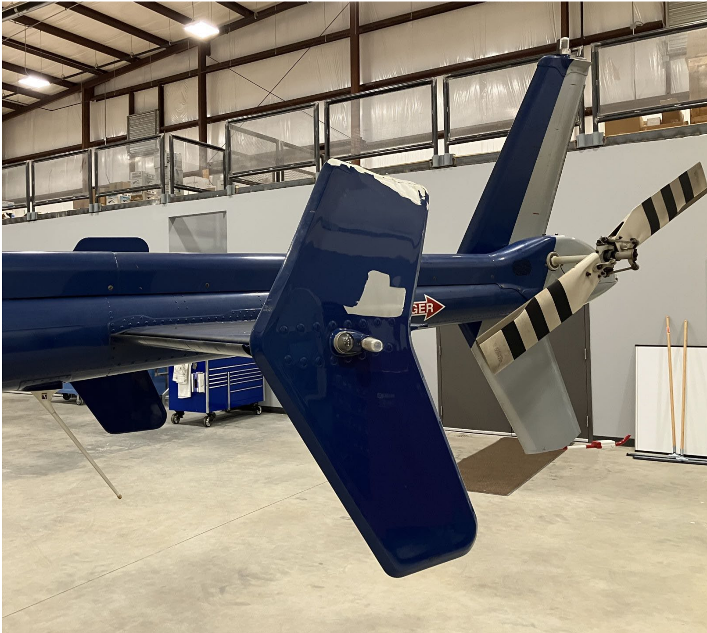
Photo 1 – View of Damaged Left Vertical Stabilizer (VSP)
