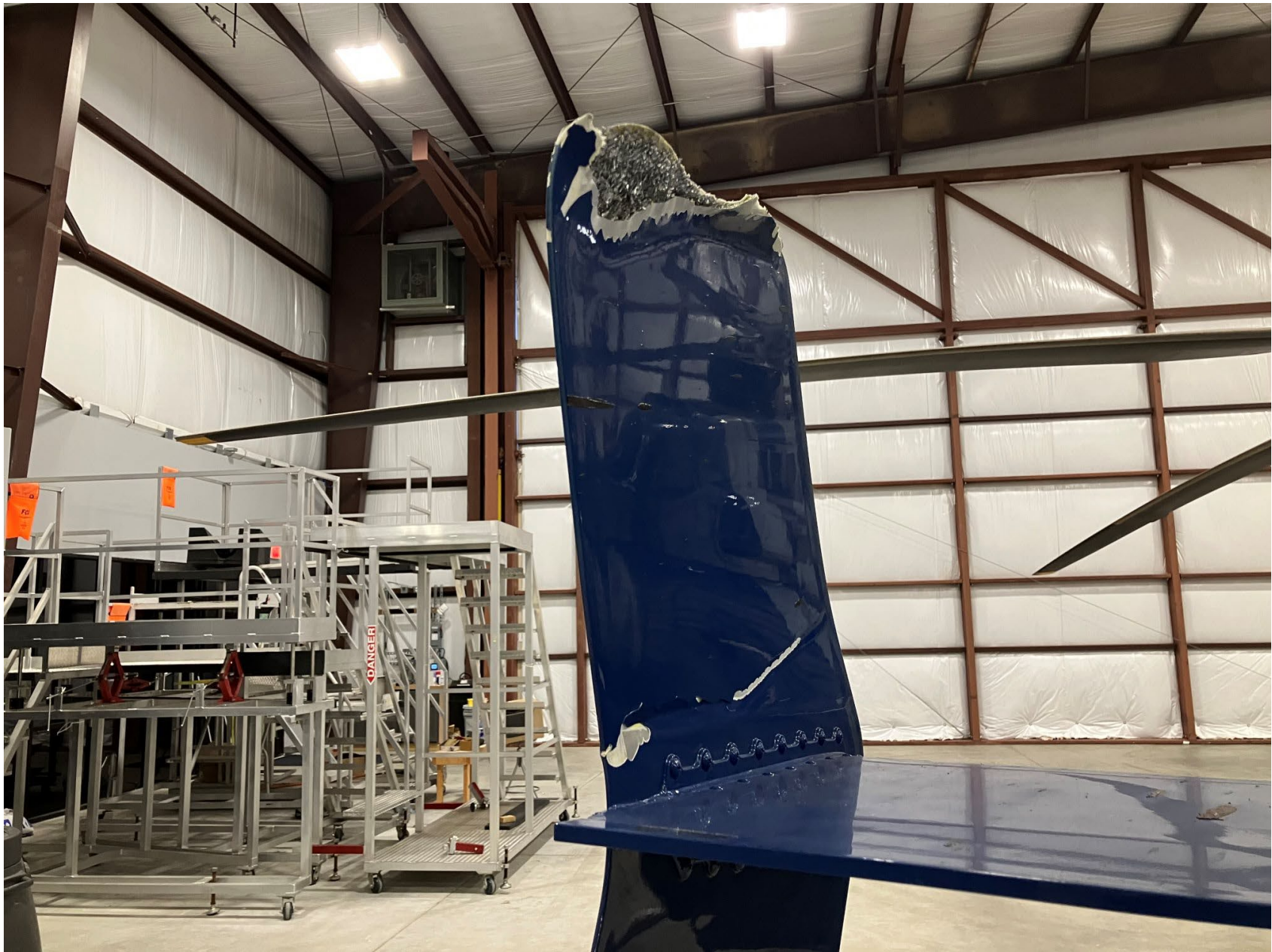
Photo 3 - View of Damaged Vertical Stabilizer Facing Opposite Direction of M/R Rotation (VSP)
