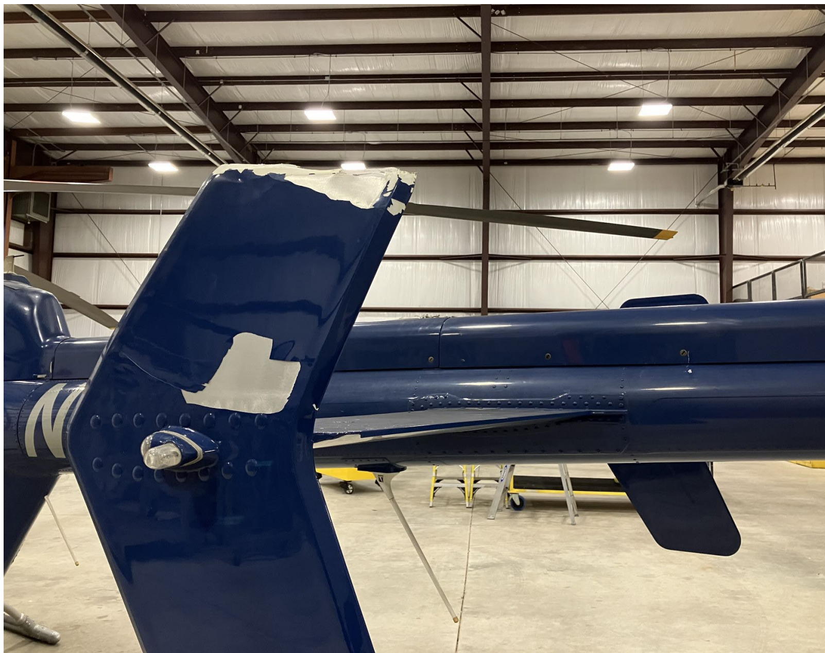
Photo 2 – View of Damaged Vertical Stabilizer Facing Direction of M/R Rotation (VSP)
