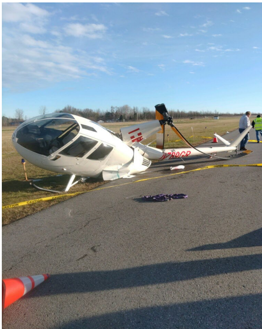
Photograph 2 - Forward view of helicopter showing hull and rotor blade damage (Courtesy of FAA)
