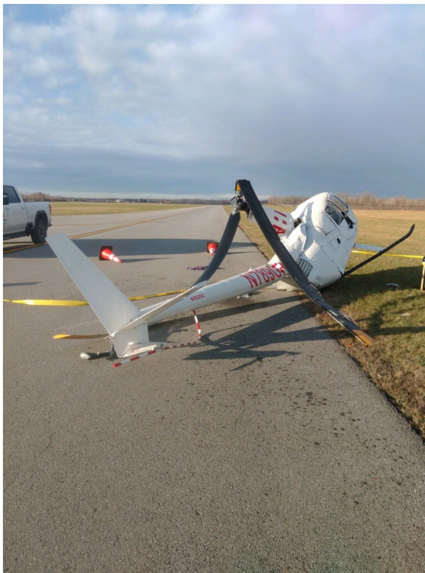
Photograph 1 - Rear view of helicopter showing tail boom damage (Courtesy of FAA)
