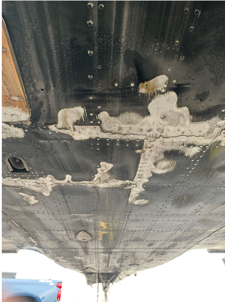
Photograph 4 - Photograph From Airport Manager. View of the Bottom Fuselage Skin. Note the Abrasion Damage.
