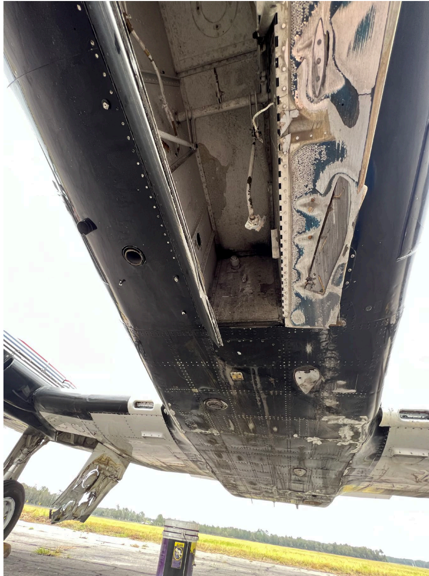
Photograph 2 - Photograph From Insurance Adjuster. View taken From the Nose Landing Gear Wheel Well Looking aft Showing the Bottom Fuselage Skin Scrape Damage
