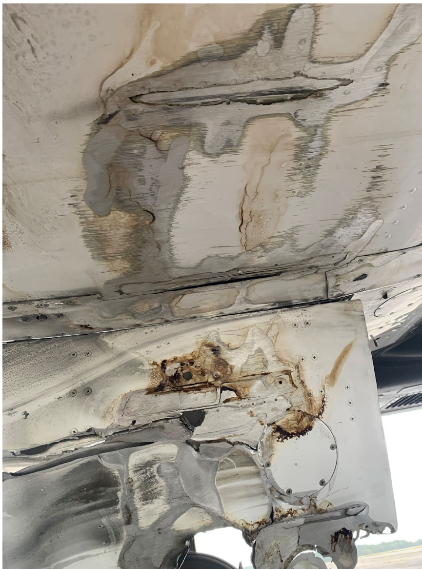
Photograph 3 - Photograph From Airport Manager. View of the Bottom Wing Skin of the Left Wing. Note the Abrasion Damage in several areas.
