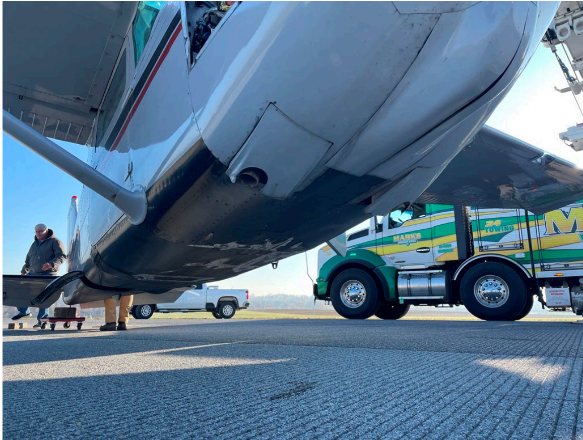
Photograph 1 - Structural Damage to Airplane Belly (Courtesy of FAA)
